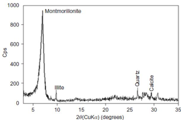
Fig. 1 X-ray diffraction plots of the Bentonite used in this study
