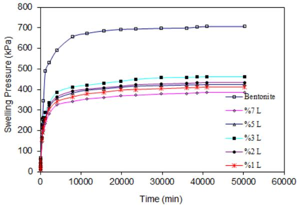
Fig. 3 Swelling pressure versus time for bentonite-lime mixture
