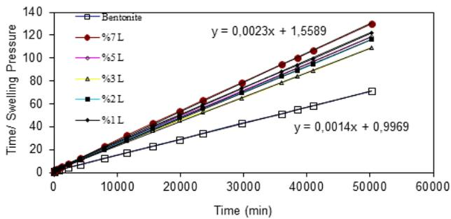
Fig. 7 Time/swelling pressure versus time for Bentonite-lime mixture
