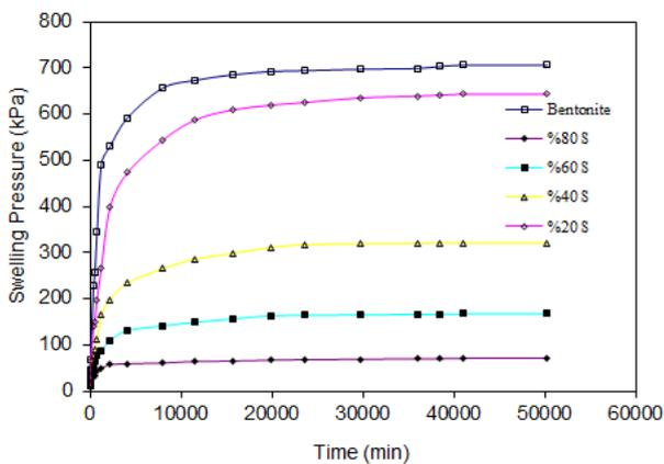
Fig. 4 Swelling pressure versus time for bentonite-sand mixture
