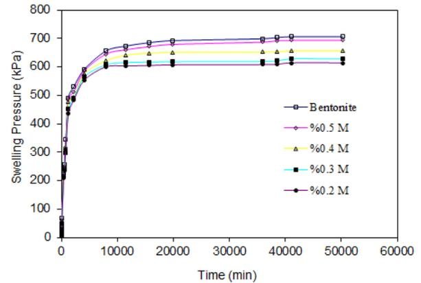
Fig. 5 Swelling pressure versus time for bentonite-multifilament fiber mixture
