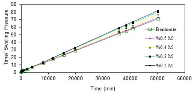
Fig. 9 Time/swelling pressure versus time for Bentonite-multifilament fiber mixture
