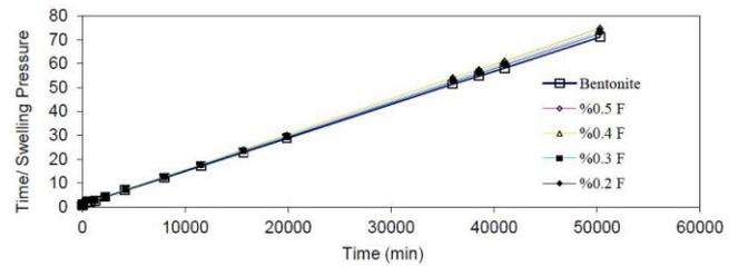
Fig. 10 Time/swelling pressure versus time for Bentonite-fibrillated fiber mixture
