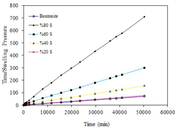
Fig. 8 Time/swelling pressure versus time for Bentonite-sand mixture
