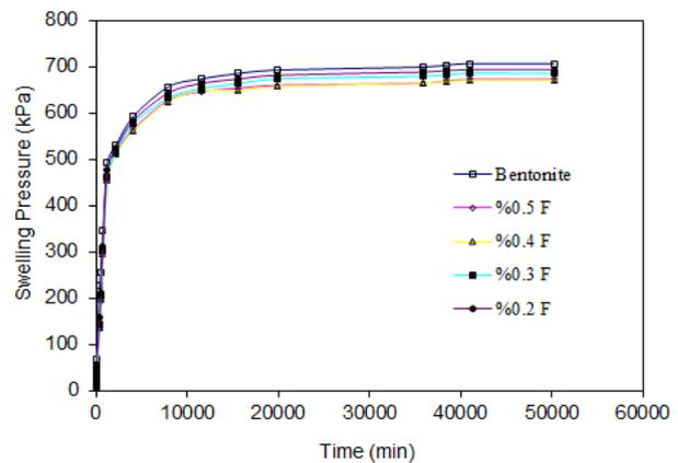
Fig. 6 Swelling pressure versus time for bentonite-fibrillated fiber mixture
