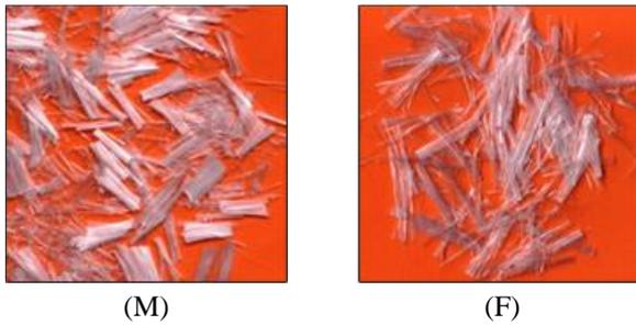
Fig. 2 Multifilament fiber (M) and fibrillated fiber (F) used in this study (as supplied by the manufacturer)
