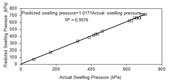
Fig. 11 Actual swelling pressure vs. predicted swelling pressure for all the test results
