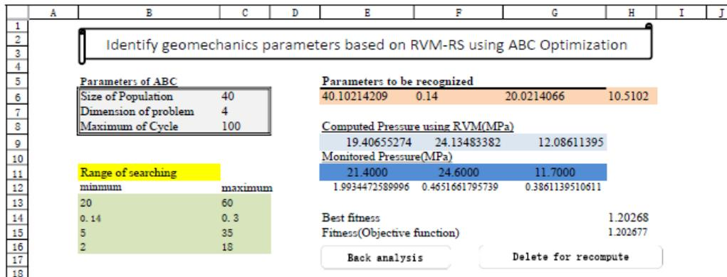
Fig. 6 The worksheet of hybrid back analysis using ABC
