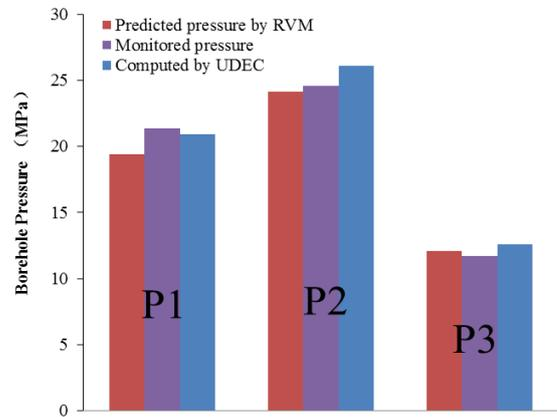
Fig. 7 The comparison pressure based on different method
