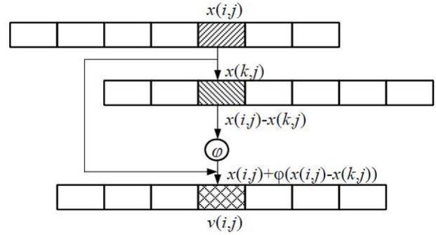
Fig. 1 Illustrating a simple position update equation execution
