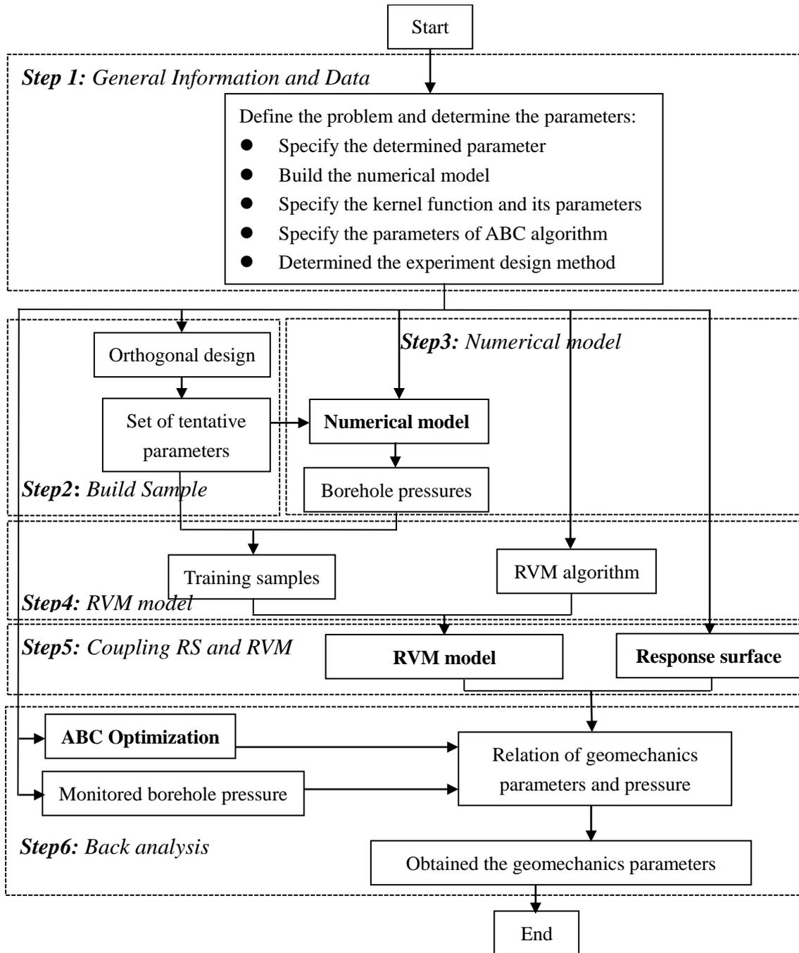
Fig. 2 The flowchart of the proposed method
