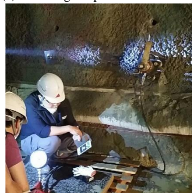
Fig. 5 Rock bolt pullout test
