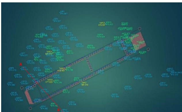
Fig. 6 Layout of surface settlement monitoring points layout of Line 2
