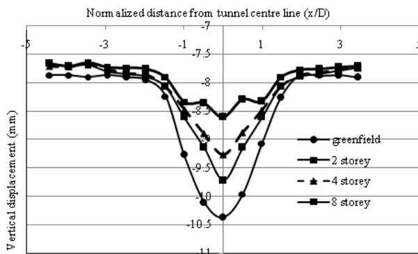
Fig. 3 Displacements on surface with building placed on centre line of the tunnel
