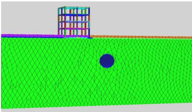
Fig. 2 Meshed model with building placed at 10 m from centre line
