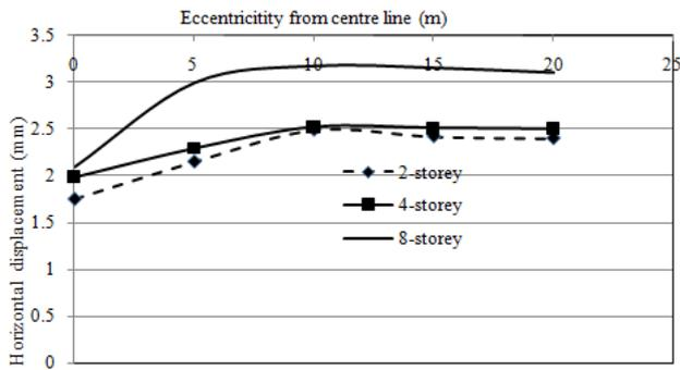
Fig. 8 Displacements on surface with 2, 4, 8-storey building placed at varying eccentricities from centre line
