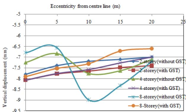
Fig. 10 Displacement under footing with varying building eccentricity and storeys
