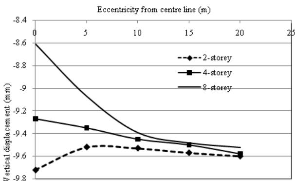
Fig. 4 Displacements on surface with 2, 4, 8-storey building placed at varying eccentricities from centre line
