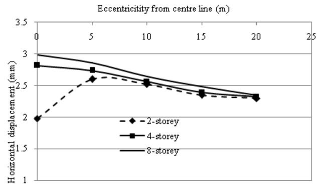
Fig. 5 Horizontal displacement along depth with varying building eccentricity and storey
