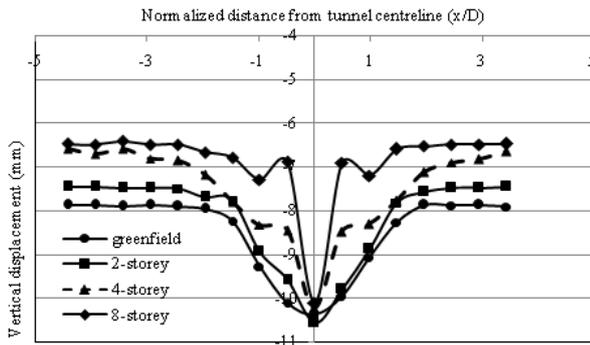
Fig. 6 Displacements on surface with 2, 4, 8-storey building placed on centre line
