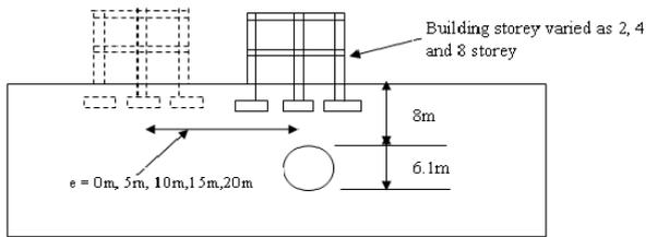
Fig. 1 Location of building with respect to tunnel
