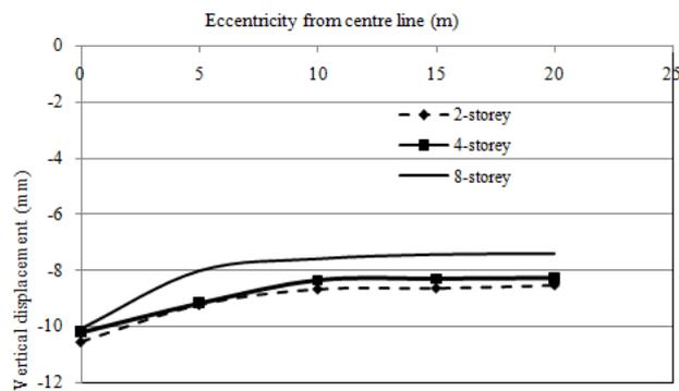
Fig. 7 Displacements on surface with 2, 4, 8-storey building placed at varying eccentricities from centre line
