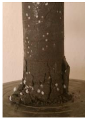
Fig. 8 Formation of local failure with increase of EPS content
