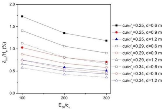
Fig. 4 Effect of soil stiffness on normalized wall deflection for  $H_e=20$  m,  $\gamma=17$  kN/m<sup>3</sup>,  $B=30$  m and  $T=30$  m)
