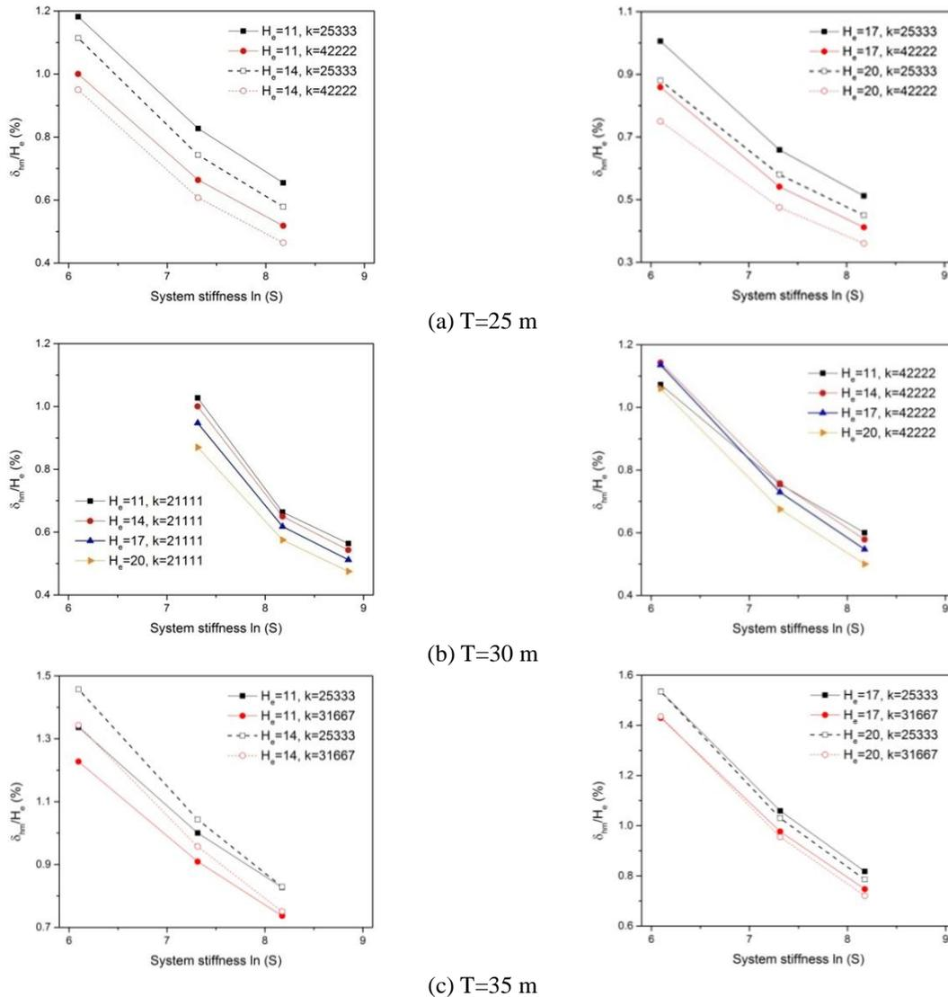
Fig. 6 Effect of excavation depth  $H_e$  on normalized wall deflection for (a)  $T=25$  m, (b)  $T=30$  m and (c)  $T=35$  m ( $c_u/\sigma'_v=0.29$ ,  $E_{50}/c_u=200$ , and  $\gamma=17$  kN/m<sup>3</sup>)
