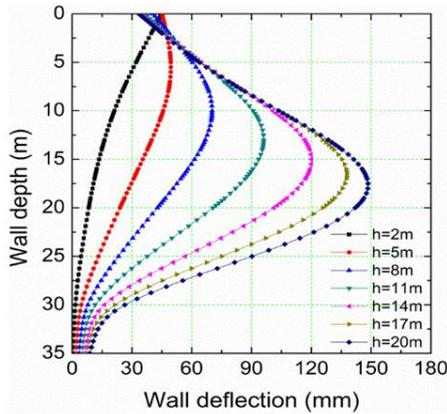
Fig. 3 Wall deflection profile for different excavation stage
