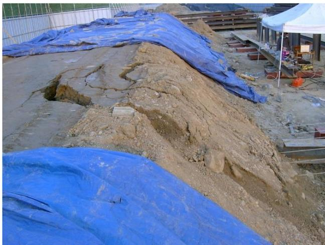
Fig. 7 Tension crack occurred in test embankment during the pullout test
