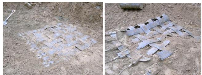
(a) 6×6 treadmat failed by pullout (b) 6×6 treadmat failed by breakage
