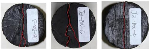
Fig. 3 Splitting failure pattern (Sample diameter=50 mm)
