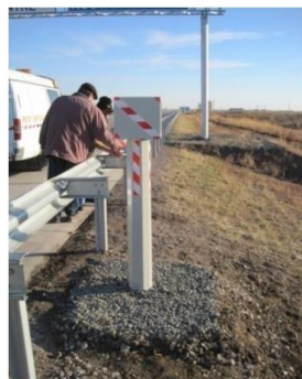
Fig. 6 Measurement (land) system for set of temperature and moisture sensors
