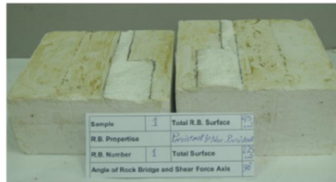
Fig. 8 Failure pattern in rock bridge configuration of “d” with area of (a) 45 cm 2 ; (b) 90 cm 2
