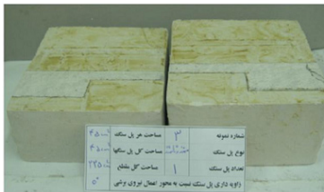
Fig. 9 Failure pattern in rock bridge configuration of “e” with area of (a) 45 cm 2 ; (b) 90 cm 2
