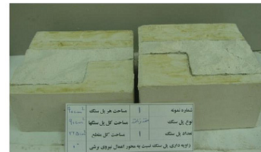
Fig. 8 Failure pattern in rock bridge configuration of “d” with area of (a) 45 cm 2 ; (b) 90 cm 2
