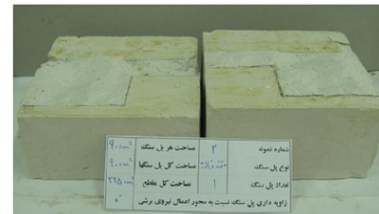
Fig. 9 Failure pattern in rock bridge configuration of “e” with area of (a) 45 cm 2 ; (b) 90 cm 2
