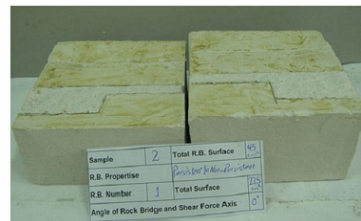
Fig. 8 Failure pattern in rock bridge configuration of “d” with area of (a) 45 cm 2 ; (b) 90 cm 2
