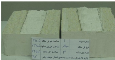
Fig. 5 Failure pattern in rock bridge configuration of “a” with area of (a) 45 cm 2 ; (b) 90 cm 2
