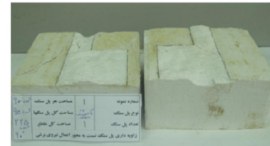
Fig. 8 Failure pattern in rock bridge configuration of “d” with area of (a) 45 cm 2 ; (b) 90 cm 2
