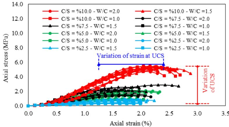
(d) Compacted with 40 MPa static pressure and cured for 28 days
