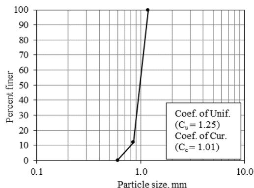
Fig. 1 Particle size distribution curve of the sand used in the study (modified from Barzegari Kahnemouei 2013)
