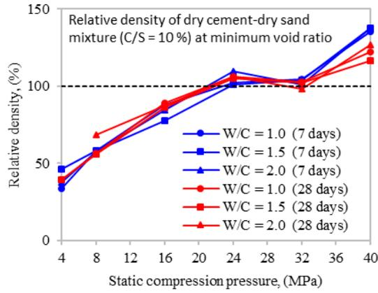
Fig. 5 Variation of relative density of the samples (C/S = 10%) with compaction pressure
