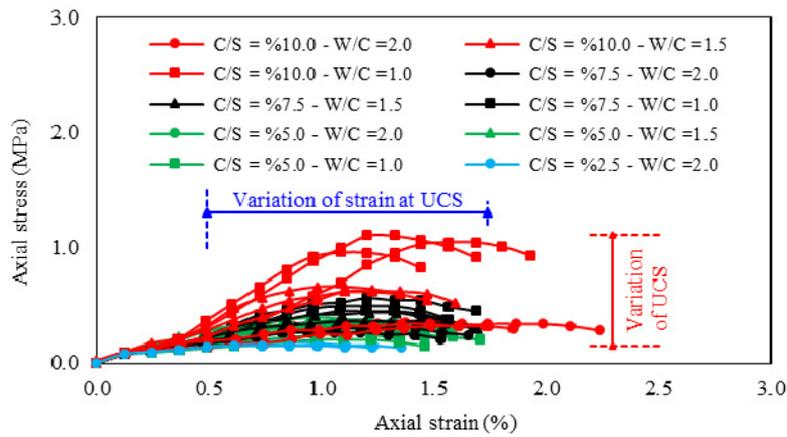
(a) Compacted with 8 MPa static pressure and cured for 7 days
