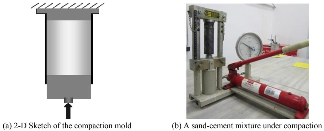
Fig. 2 Compaction mold and compaction apparatus (Barzegari Kahnemouei 2013)
