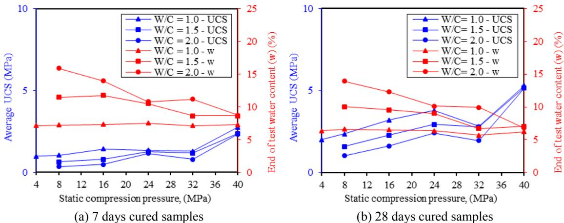
Fig. 4 Variation of average UCS and end of test water content (average) with static compaction pressure
