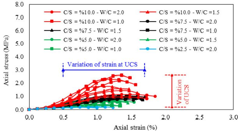
(c) Compacted with 8 MPa static pressure and cured for 28 days
