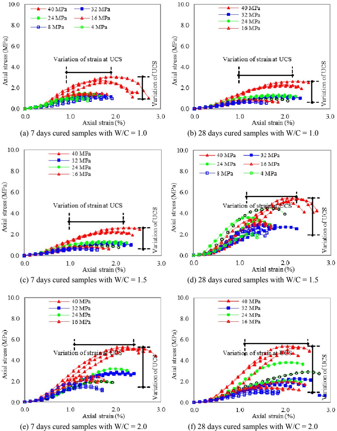
Fig. 3 Variation of axial stress-axial strain curves of the samples with C/S = 10.0%
