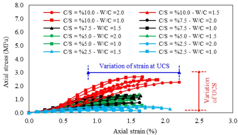
(b) Compacted with 40 MPa static pressure and cured for 7 days
