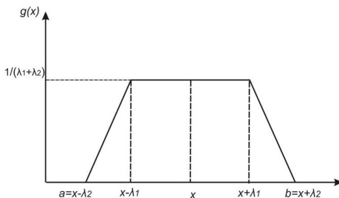
Fig. 3 Trapezoidal density function and critical parameters (BIPM 2008b)
