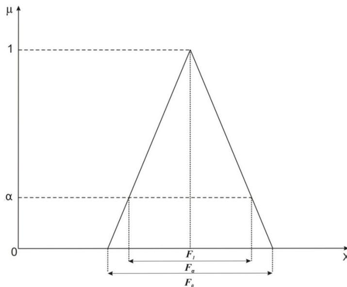
Fig. 2 A representation for triangular function and alpha-cut
