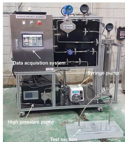
Fig. 4 Experimental setup for grout injection and permeability test
