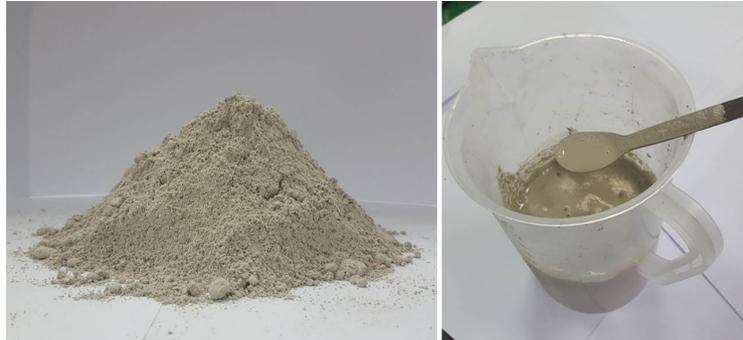
Fig. 2 Micro cement material for grouting injection
