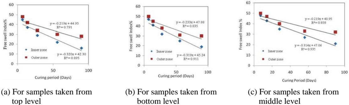
Fig. 13 Variation of free swell index with different curing periods in the inner and outer zones
