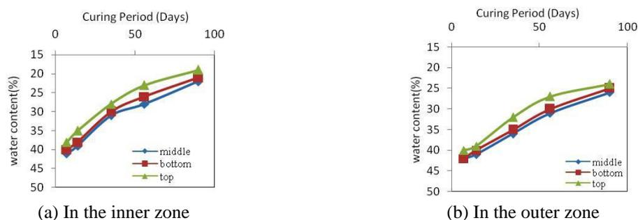
Fig. 14 Variations of water content with depths for the stabilized soil at different curing periods
