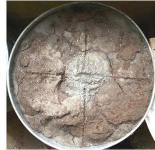
Fig. 3 Waste slurry permeating into shrinkage cracks
