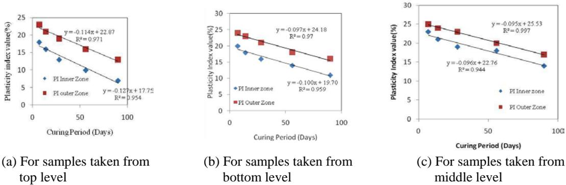
Fig. 9 Fluctuations in plasticity index (PI) values at a radial distance of 10 cm (Inner) and 20 cm (Outer) with different curing periods
