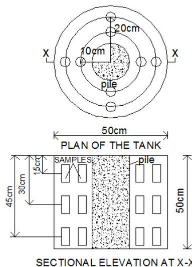
Fig. 8 Plan and Elevation of the model tank showing the sampling points
