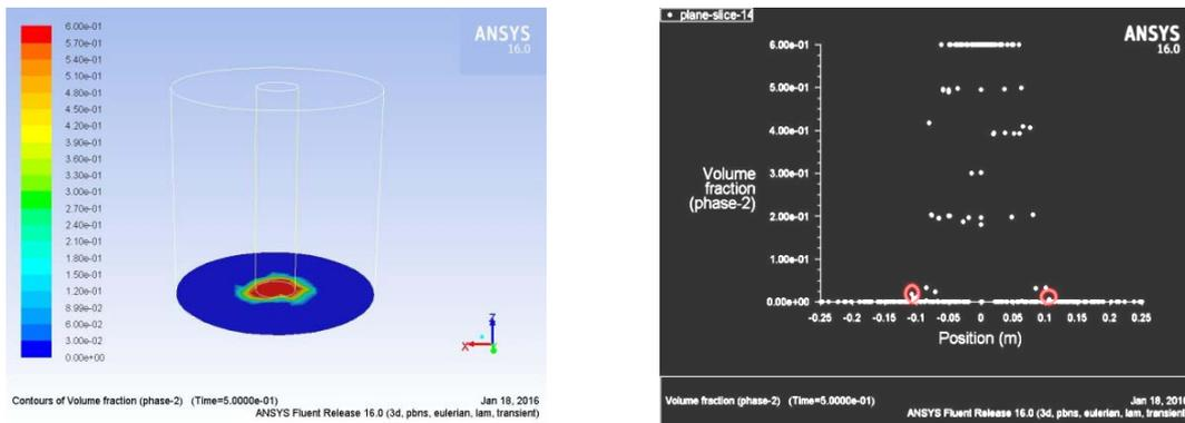
Fig. 5 Dispersion of slurry at the bottom plane section
