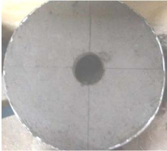
Fig. 1 Clay sample statically compacted inside the mould
