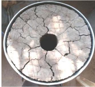
Fig. 2 Formation of shrinkage cracks
