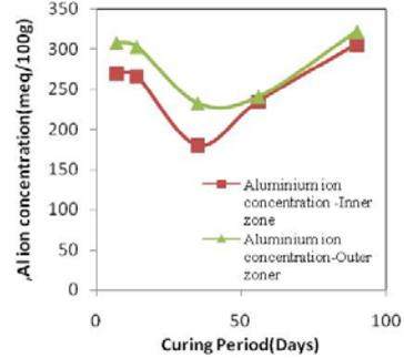
Fig. 16 Concentration of Aluminium ions at two radial distances of 10 cm, 20 cm for samples taken at top level
