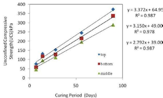
Fig. 12 Correlation between shear strength and curing period for the Outer zone at varying depths (top, middle, bottom)
