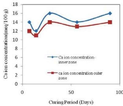
Fig. 17 Concentration of Calcium ions at two radial distances of 10 cm, 20 cm for samples taken at top level
