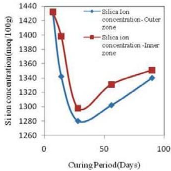
Fig. 15 Concentration of silica ions at two radial distances of 10 cm, 20 cm for samples taken at top level
