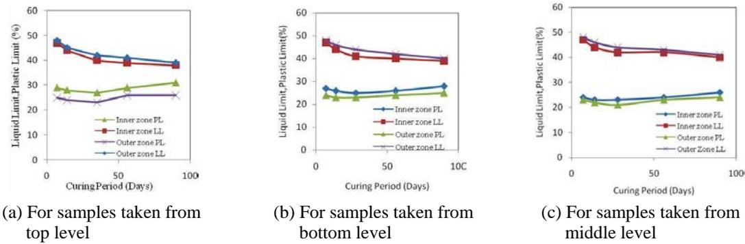
Fig. 10 Variation of Liquid limit (LL), Plastic limit (PL) in inner and outer zone with different curing periods
