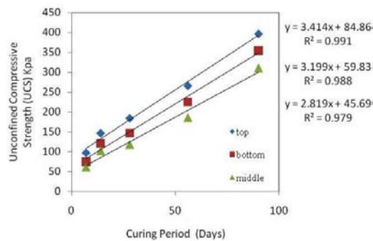
Fig. 11 Correlation between shear strength and curing period for the Inner zone at varying depths (top, middle, bottom)
