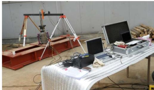
Fig. 4 Pullout test setup for measuring of pre-stress force and load transfer at construction sites
