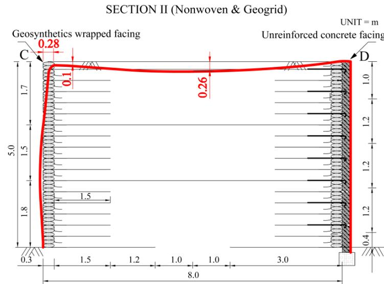
(b) External deformation at SECTION II
