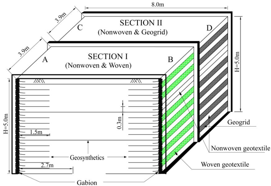
Fig. 1 Schematic diagram of GRS walls
