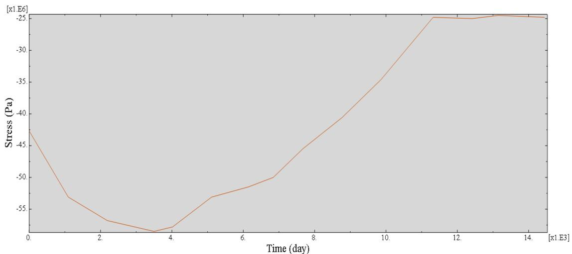
Fig. 9 The maximum principal stresses changes around the well No. 1 during production and injection scenarios
