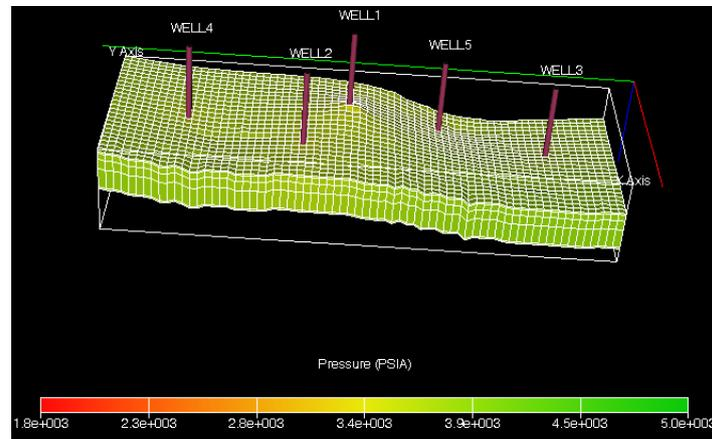
Fig. 3 Flow model: grid discretization, well system and initial pressure distribution
