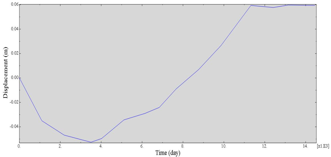
Fig. 8 Vertical displacement changes around the well No. 1 during production and injection scenarios
