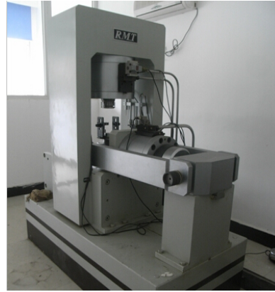
Fig. 2 Rock Mechanical Test System (RMT)
