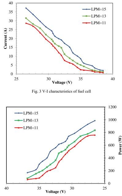
Fig. 4 Characteristics of fuel cell at different flow rate of hydrogen
