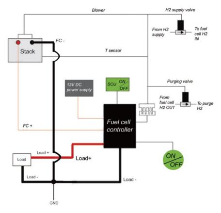
Fig. 2 System setup diagram
