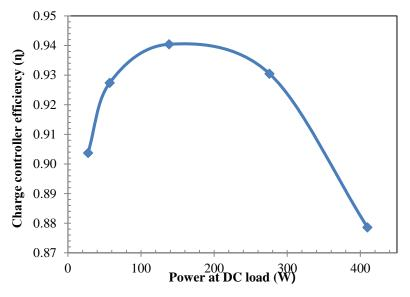
Fig. 5 Power at DC load vs Charge controller efficiency
