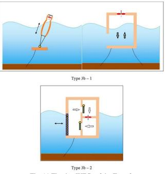
Fig. 11 Floating WECs of the Type 3
