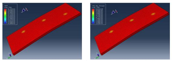
Fig. 11 Reservoir temperature distribution (left) and related maximum thermal strain (right)
