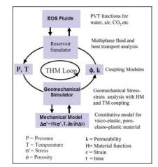
Fig. 3 THM loop (linking between ECLIPSE and ABAQUS)
