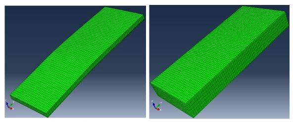
Fig. 2 3D geomechanical model: reservoir (left), and reservoir and its surrounding (right)
