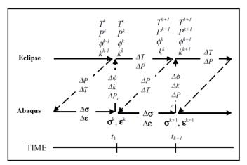
Fig. 4 Explicit sequential solutions of a linked ECLIPSE and ABAQUS simulation
