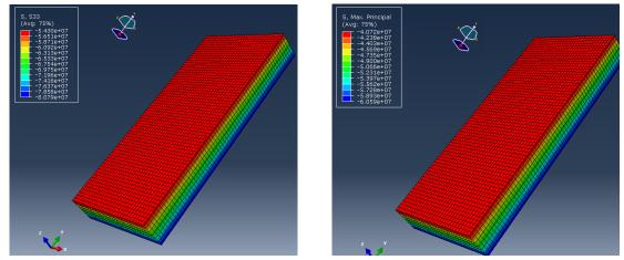
Fig. 10 Vertical stress (left), and maximum principal stress (right) distribution
