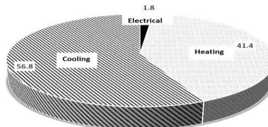
Fig. 4 Percent use of annual cooling, heating and electrical loads for rural villa through a year
