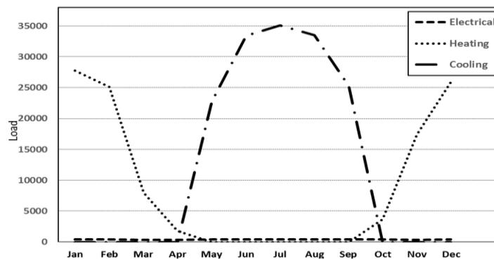
Fig. 3 Monthly average consumption rate of electrical, heating and cooling loads for rural villa on the fifteenth day of December
