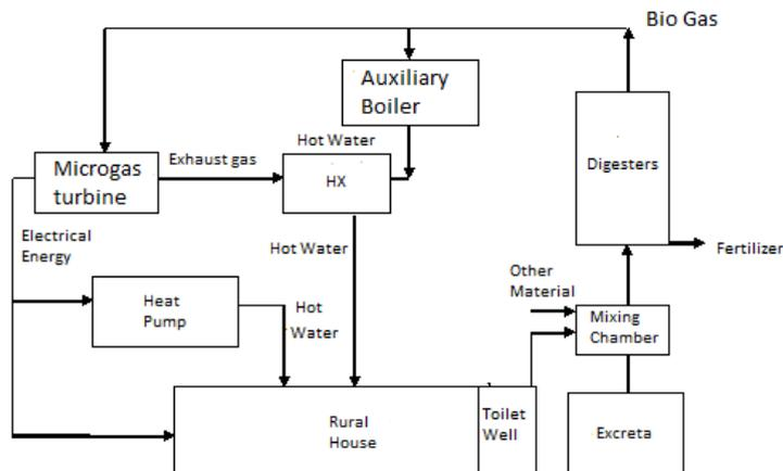
Fig. 6 A schematic of method to supply the energy needed by the rural house using biogas-fueled microturbine in winter
