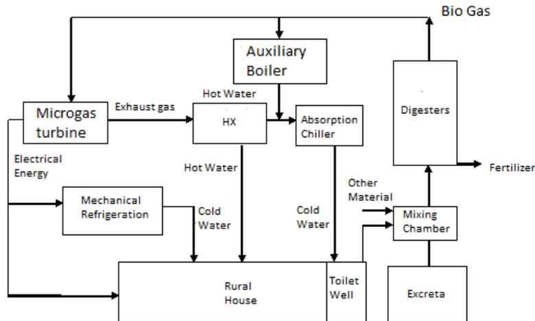
Fig. 5 A schematic of method to supply the energy needed by the rural house using biogas-fueled microturbine in summer
