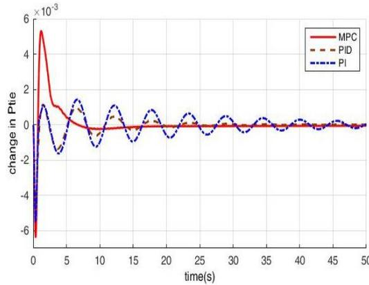
Fig. 21 Change in  $P_{tie}$  for 5% step increment in  $P_{L2}$
