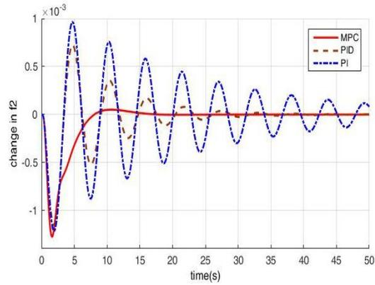
Fig. 20 Change in  $f_2$  for 5% step increment in  $P_{L2}$
