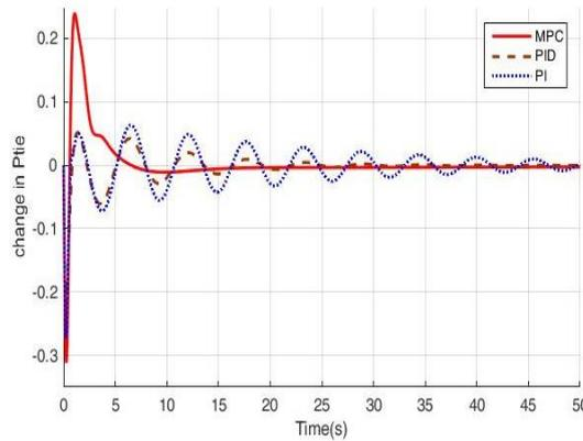
Fig. 18 Change in  $P_{tie}$  for 5% step increment in  $P_{L1}$
