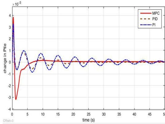
Fig. 15 Change in  $P_{tie}$  for -3% step increment in  $P_{L2}$
