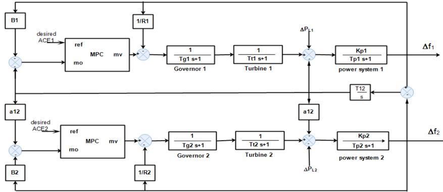
Fig. 3 Proposed two-area LFC scheme by using MPC
