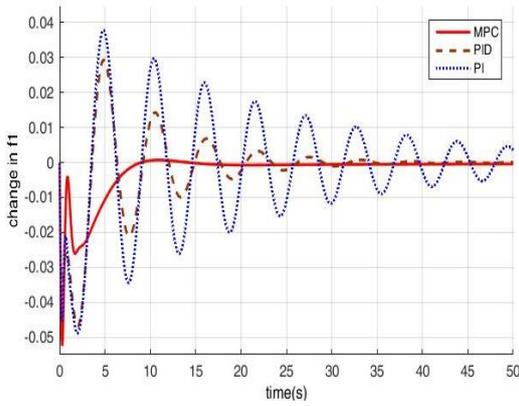
Fig. 16 Change in  $f_1$  for 5% step increment in  $P_{L1}$
