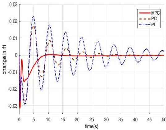
Fig. 4 Change in  $f_1$  for 3% step increment in  $P_{L1}$
