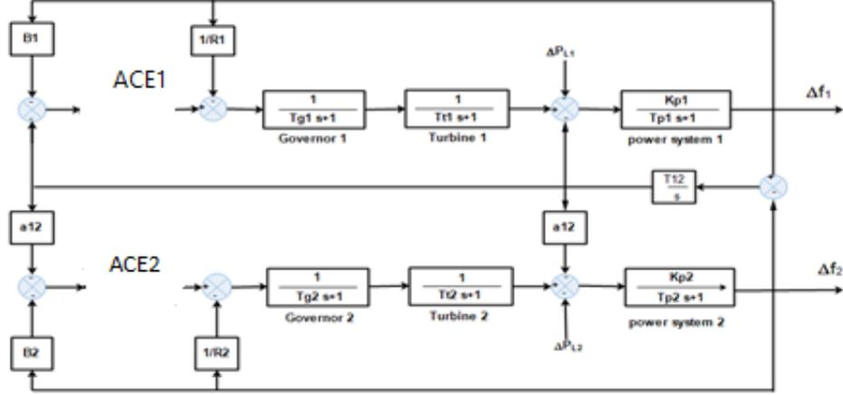
Fig. 1 Two-area interconnected power system
