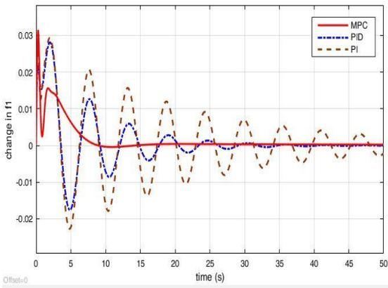
Fig. 10 Change in  $f_1$  for -3% step increment in  $P_{L1}$
