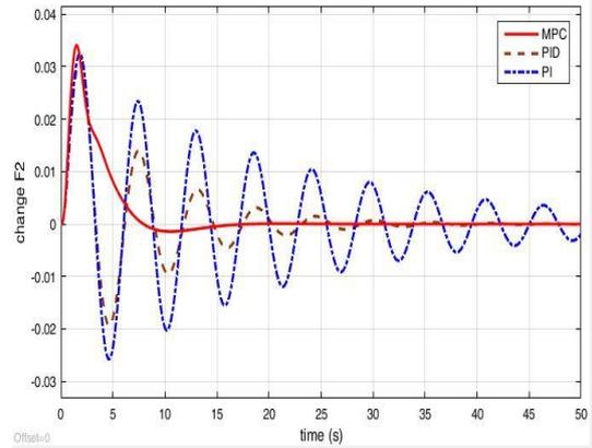
Fig. 11 Change in  $f_2$  for -3% step increment in  $P_{L1}$
