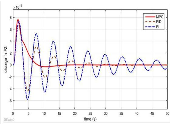
Fig. 14 Change in  $f_2$  for -3% step increment in  $P_{L2}$
