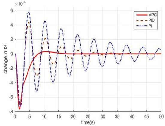
Fig. 8 Change in  $f_2$  for 3% step increment in  $P_{L2}$
