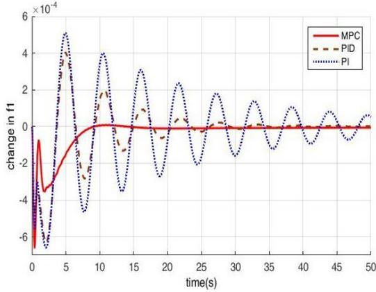
Fig. 7 Change in  $f_1$  for 3% step increment in  $P_{L2}$
