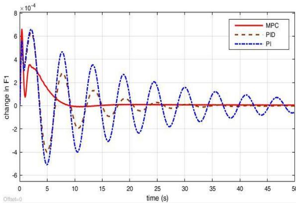
Fig. 13 Change in  $f_1$  for -3% step increment in  $P_{L2}$
