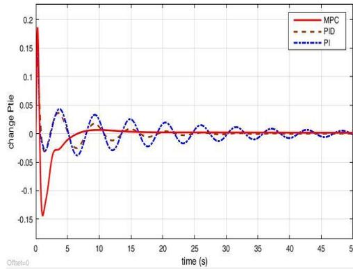
Fig. 12 Change in  $P_{tie}$  for -3% step increment in  $P_{L1}$
