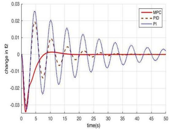
Fig. 5 Change in  $f_2$  for 3% step increment in  $P_{L1}$
