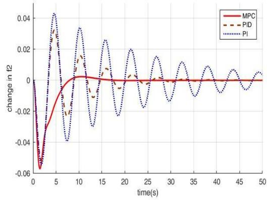
Fig. 17 Change in  $f_2$  for 5% step increment in  $P_{L1}$
