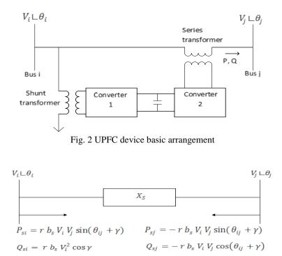
Fig. 3 UPFC injection model
