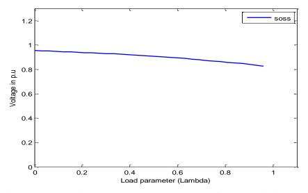
Fig. 10 P-V curve of the weakest bus (sequential UPFC) for single objective case
