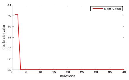
Fig. 9 Performance of SOS algorithm (sequential UPFC) for single objective case
