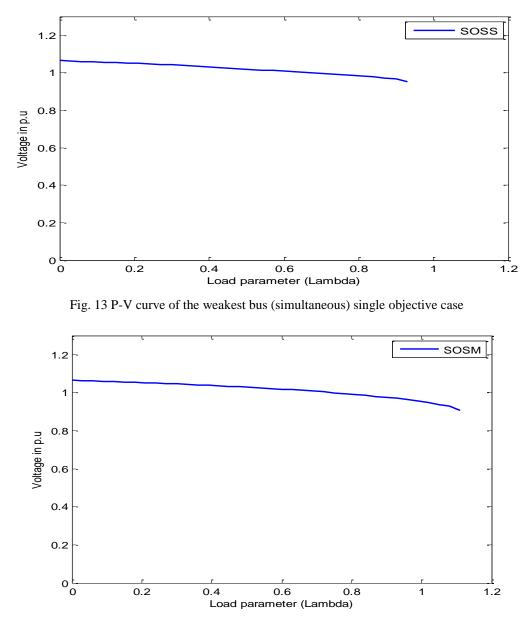
Fig. 14 P-V curve of the weakest bus (simultaneous) multi-objective case
