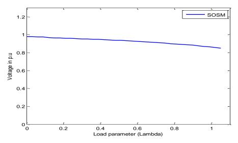
Fig. 11 P-V curve of the weakest bus (sequential UPFC) for multi-objective case
