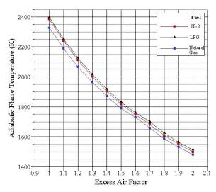
Fig. 8 The change of the adiabatic flame temperature in different excess air factor values
