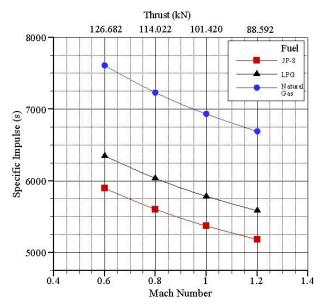
Fig. 5 The change of the specific impulse in different Mach numbers and thrust values
