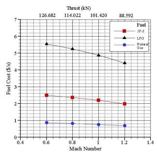
Fig. 7 The change of the fuel cost in different Mach numbers and thrust values
