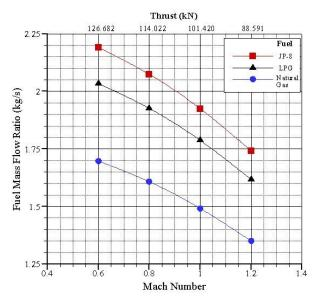
Fig. 4 The change of the fuel mass flow rate in different Mach numbers and thrust values
