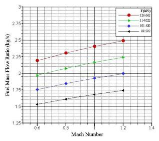
Fig. 3 The change of the fuel mass flow rate in different Mach numbers
