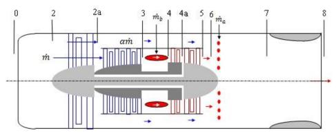
Fig. 1 Schematic view of turbofan engine with low bypass ratio; 0-2 intake, 2-2a; fan, 2a-3 high pressure compressor, 3-4 combustion chamber, 4-4a high pressure turbine, 4a-5 low pressure turbine, 5-6 mixer, 6-7 afterburner, 7-8 exhaust nozzle
