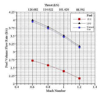
Fig. 6 The change of the fuel volume flow rate in different Mach numbers and thrust values
