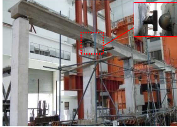
Fig. 1 Elevation view of 1/10-scale bridge model
