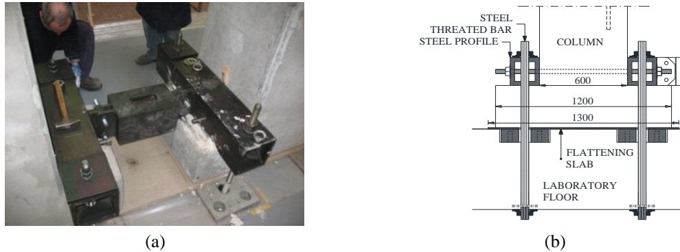
Fig. 3 Connection of the column base with the laboratory floor
