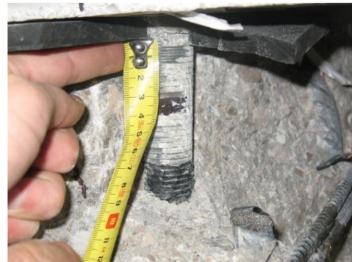
Fig. 30 Detection of the plastic hinge in one of the two steel dowels in the column at the end of monotonic test
