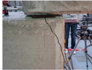
Fig. 13 Splitting of the column lateral cover (West side)
