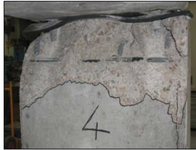
Fig. 20 Splitting of the cover at the end of the test
