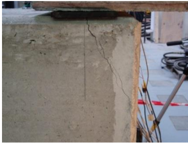
Fig. 12 First crack in the column lateral cover (West side)
