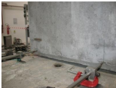
Fig. 17 Crack opening in the beam frontal cover
