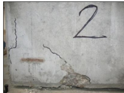
Fig. 18 Crack in the beam at the end of the test
