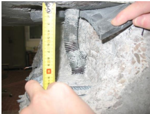
Fig. 29 Detection of the plastic hinge in one of the two steel dowels in the column at the end of cyclic test
