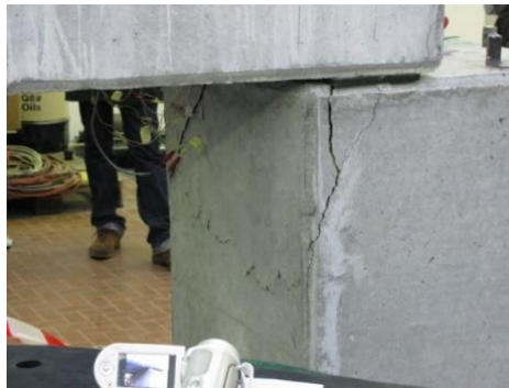
Fig. 26 Final step of the monotonic test: splitting of the concrete
