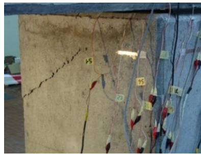
Fig. 16 Crack opening in the column frontal cover
