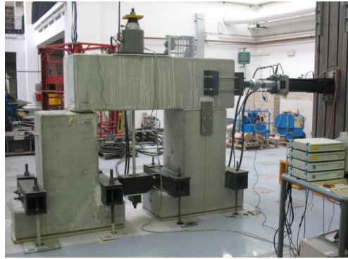
Fig. 24 Experimental setup of the monotonic shear test on a beam-to-column dowel connection
