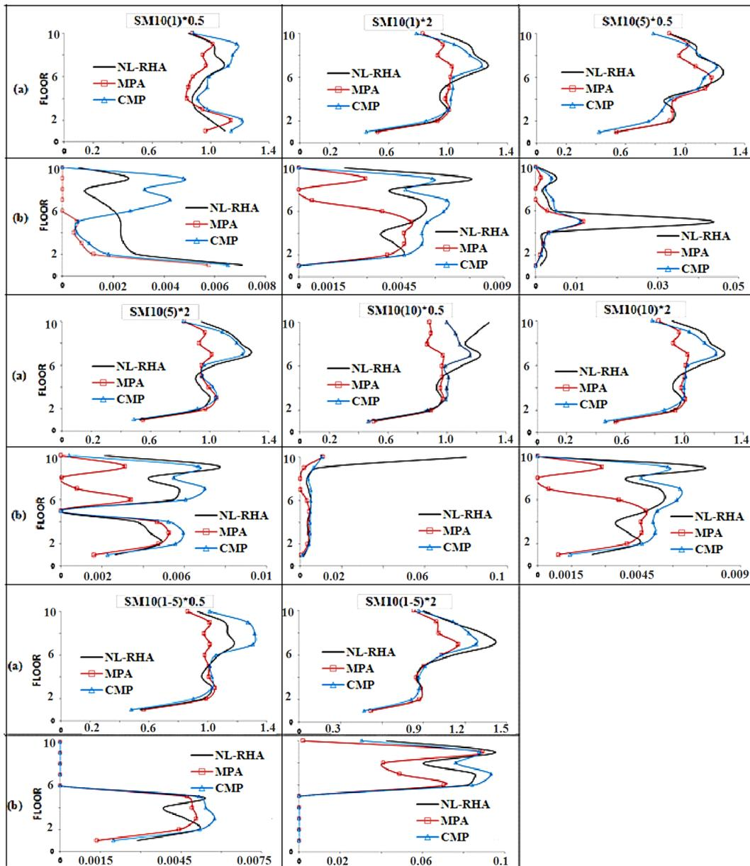
Fig. 6 Seismic responses obtained by the MPA, CMP and NL-RHA for the strength-irregular 10-storey frames: (a) storey drift ratios (%); and (b) plastic hinge rotations (rad)
