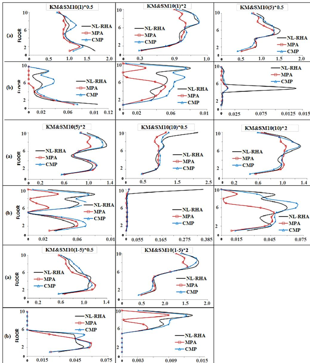
Fig. 7 Seismic responses obtained by the MPA, CMP and NL-RHA for the combined-stiffness-and-strength-irregular 10-storey frames: (a) storey drift ratios (%); and (b) plastic hinge rotations (rad)
