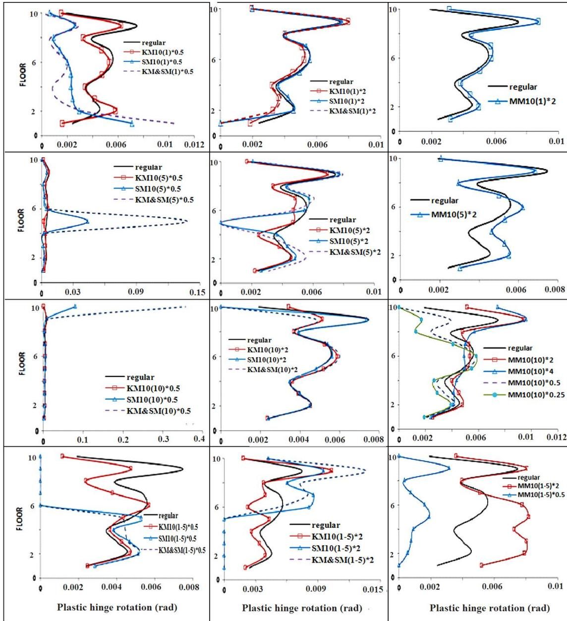
Fig. 4 Plastic hinge rotations (rad) obtained by NL-RHA for the stiffness, strength, combined-stiffness-and-strength and mass-irregular 10-storey frames denoted by *KM*, *SM*, *KM&SM* and *MM*, respectively, with modification factor, MF=2
