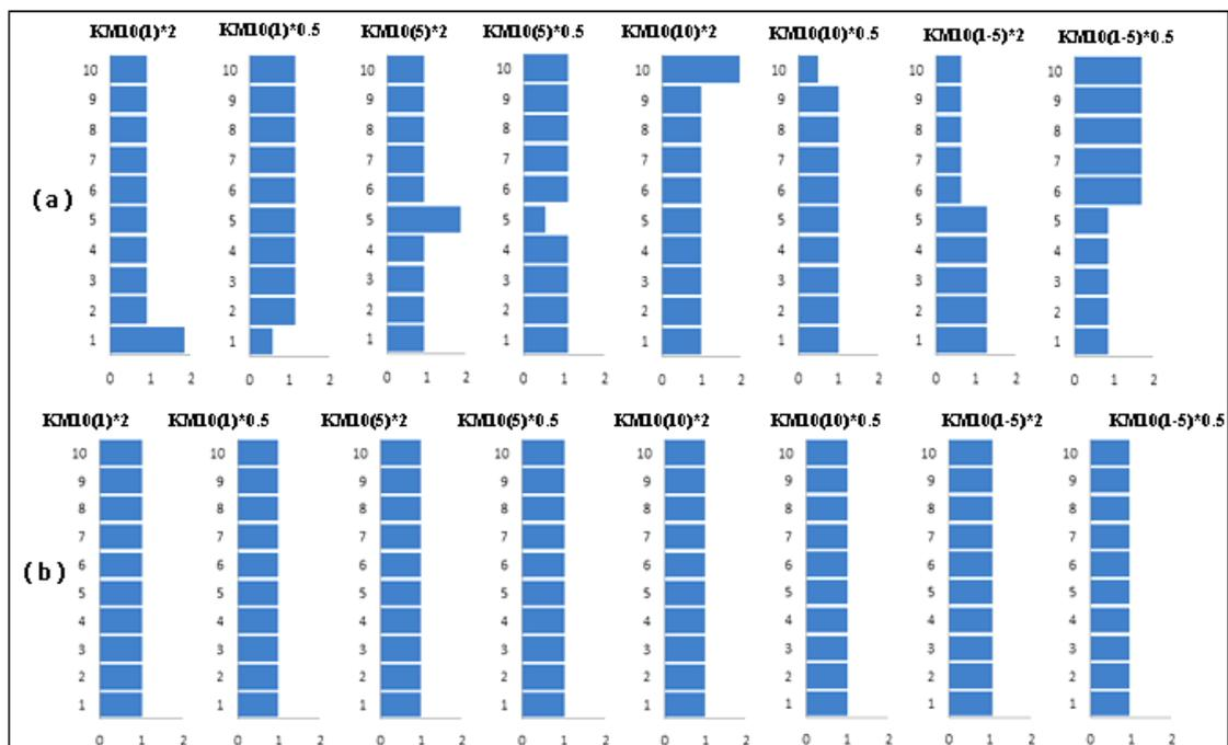
Fig. 2 Ratio of (a) storey stiffness and of (b) storey strength of the stiffness-irregular 10-storey frames to the corresponding properties of the reference regular frame for modification factor, MF=2
