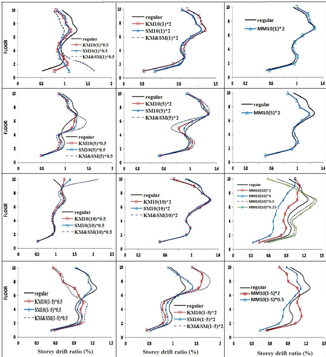
Fig. 3 Storey drift ratios (%) determined by NL-RHA for the stiffness, strength, combined-stiffness-and-strength and mass irregular 10-storey frames denoted by *KM*, *SM*, *KM&SM* and *MM*, respectively, with modification factor, MF=2
