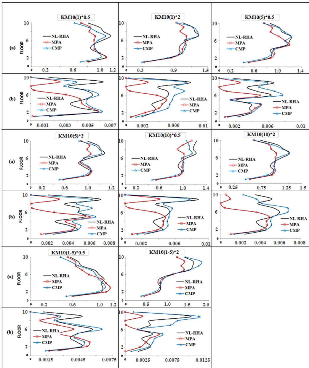
Fig. 5 Seismic responses obtained by the MPA, CMP and NL-RHA for the stiffness-irregular 10-storey frames: (a) storey drift ratios (%); and (b) plastic hinge rotations (rad)
