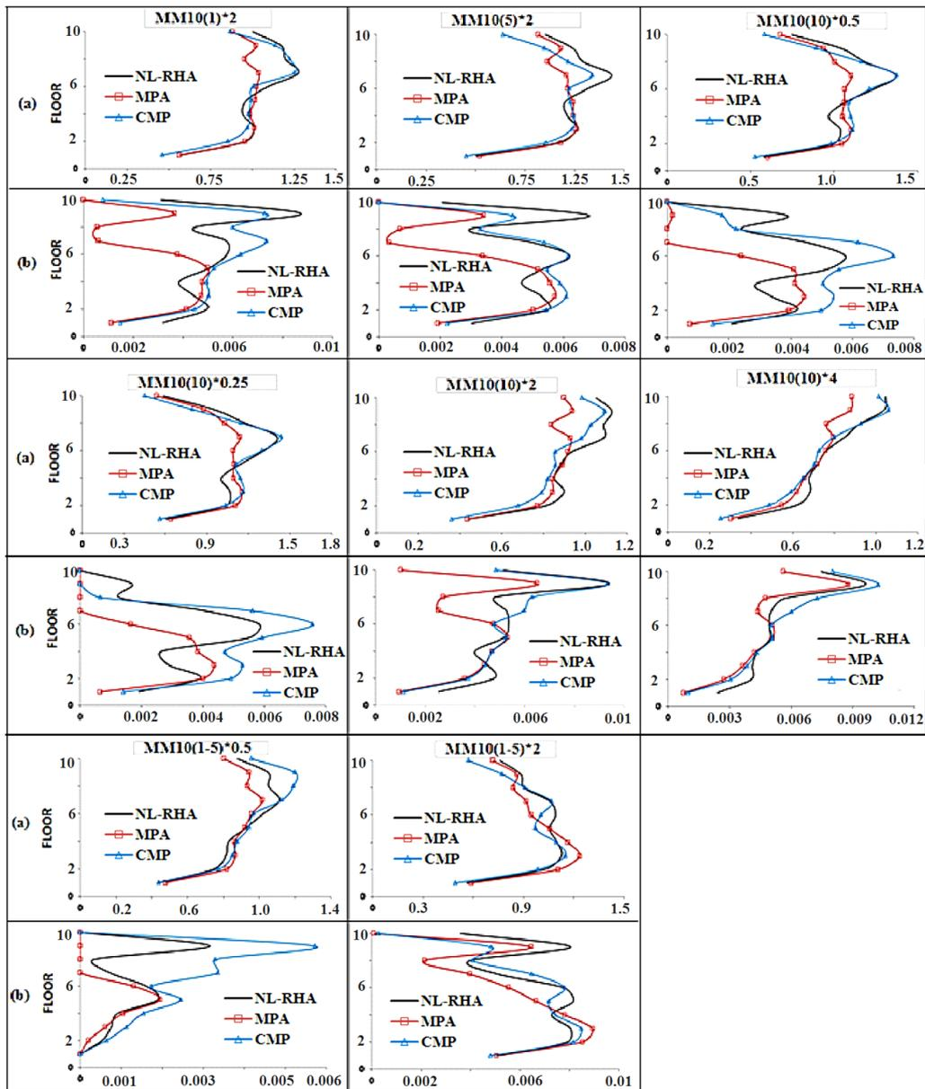
Fig. 8 Seismic responses obtained by the MPA, CMP and NL-RHA for the mass-irregular 10-storey frames: (a) storey drift ratios (%); and (b) plastic hinge rotations (rad)
