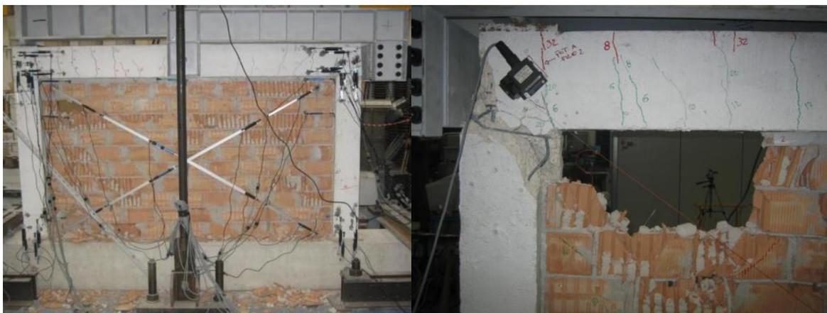
Fig. 20 Portal  $F_{11}$ : masonry crushing damage (left) and portal collapse (right)
