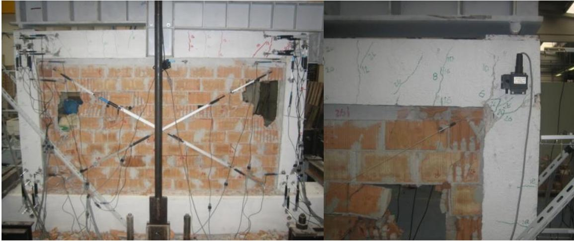
Fig. 21 Portal  $F_{12}$ : masonry crushing damage (left) and portal collapse (right)
