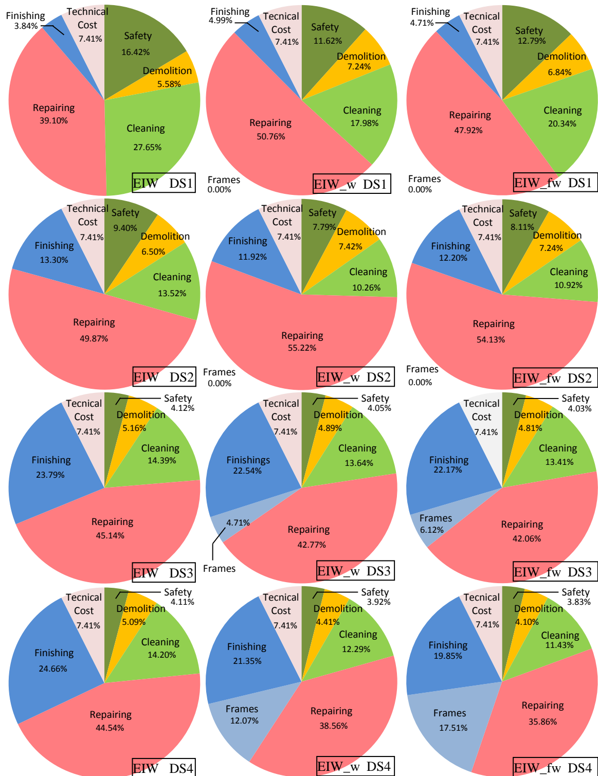
Fig. 6 Disaggregation of total repair cost ratios for infill masonry walls with and without openings
