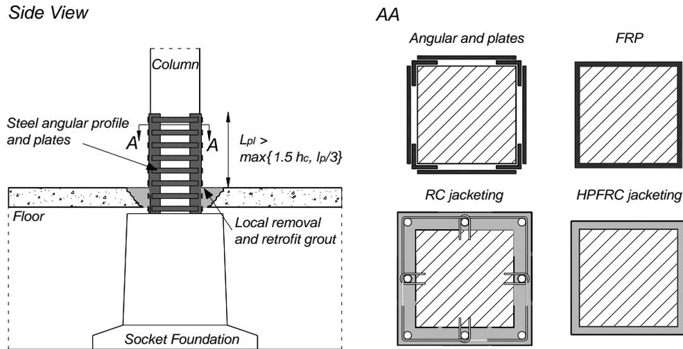
Fig. 5 Column strengthening solutions
