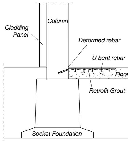
Fig. 6 Floor to column connection
