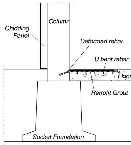
Fig. 6 Floor to column connection
