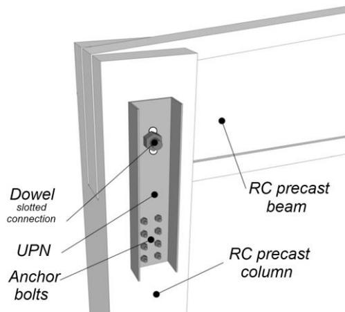
Fig. 3 Column to beam mechanical connection
