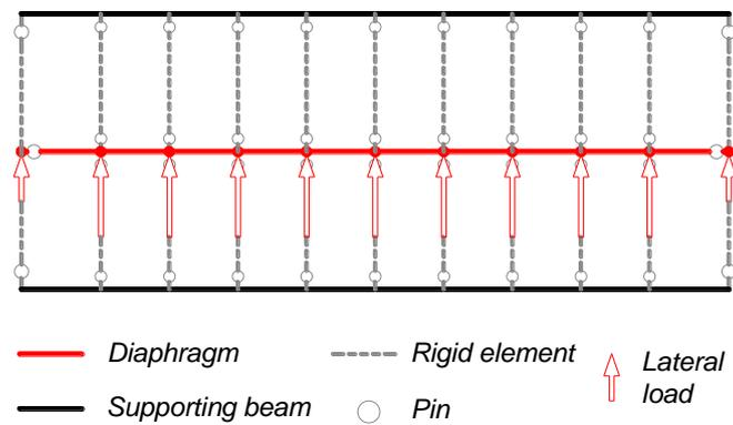
Fig. 2 Diaphragm finite element model for stiffness evaluation
