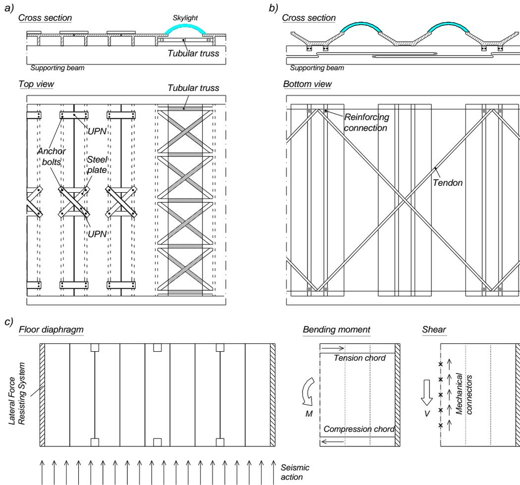
Fig. 1 Diaphragm stiffening solution: (a) double-T beams and (b) open-shape beams
