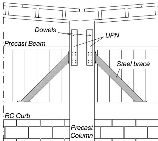
Fig. 4 Short column strengthening solutions
