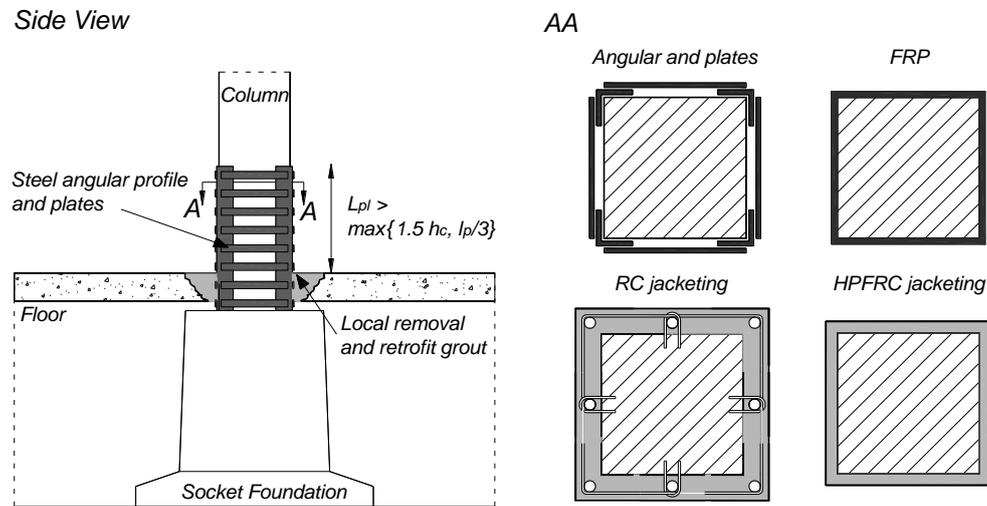
Fig. 5 Column strengthening solutions
