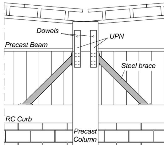
Fig. 4 Short column strengthening solutions
