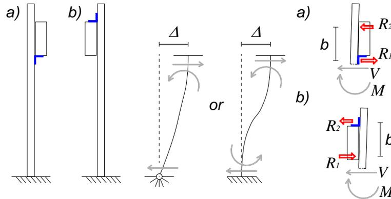
Fig. 8 Connection load demand due to out-of-plane displacement of vertical cladding panel
