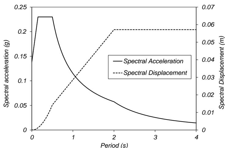
Fig. 10 Acceleration and displacement reference spectrum
