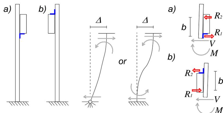
Fig. 8 Connection load demand due to out-of-plane displacement of vertical cladding panel
