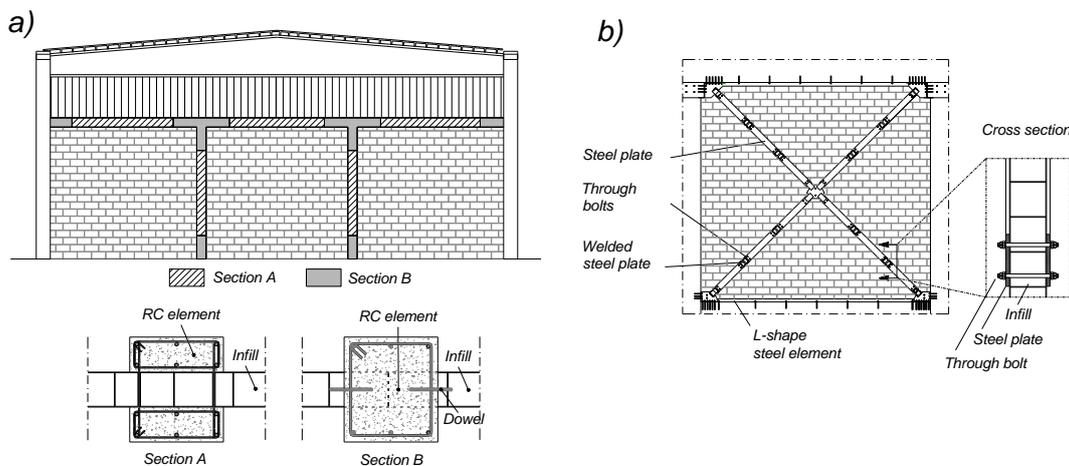
Fig. 7 Infill capacity retrofit solutions: (a) out-of-plane, (b) in-plane
