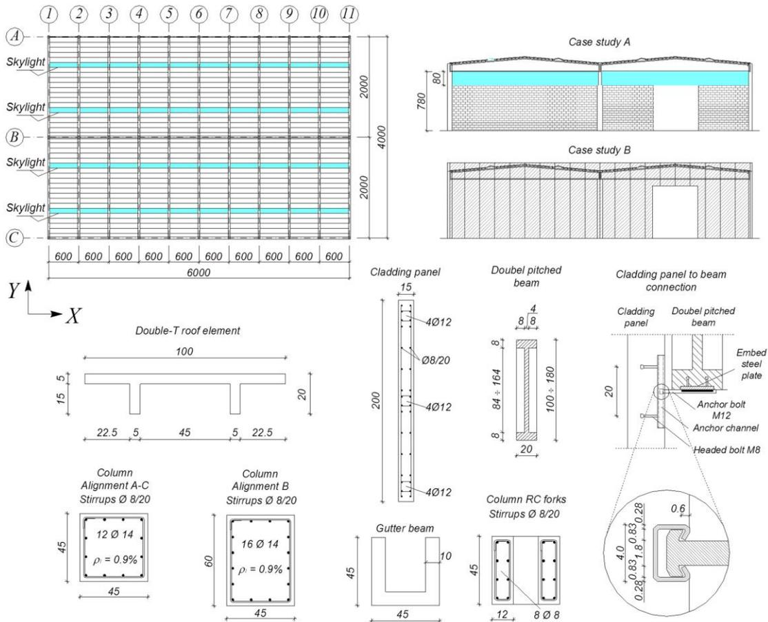
Fig. 9 Building geometry relevant data (measures in cm)
