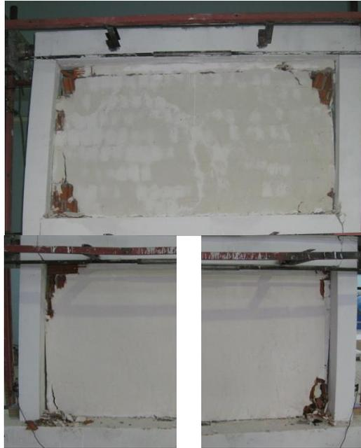
Fig. 8 Failure modes of the wall portions (Korkmaz *et al.* 2010)
