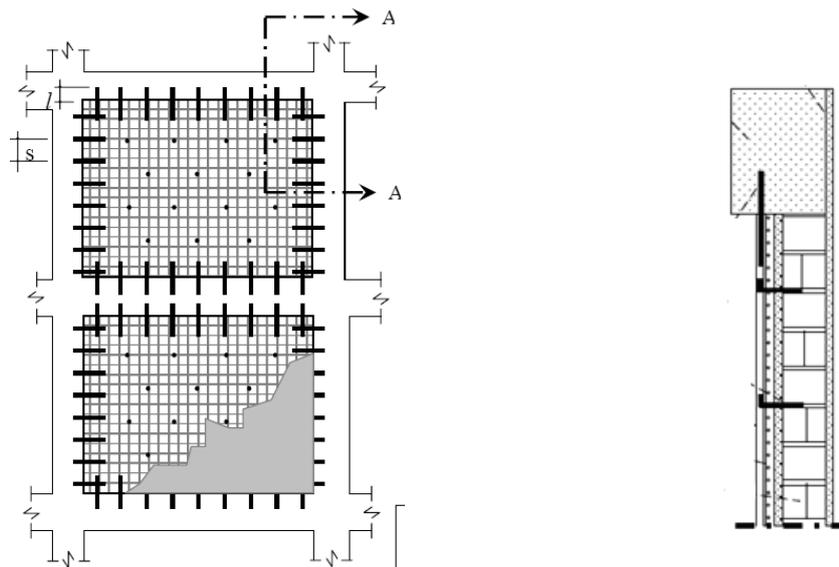
Fig. 4 Plastered wall with welded external mesh and plaster composite (TEC-2007)
