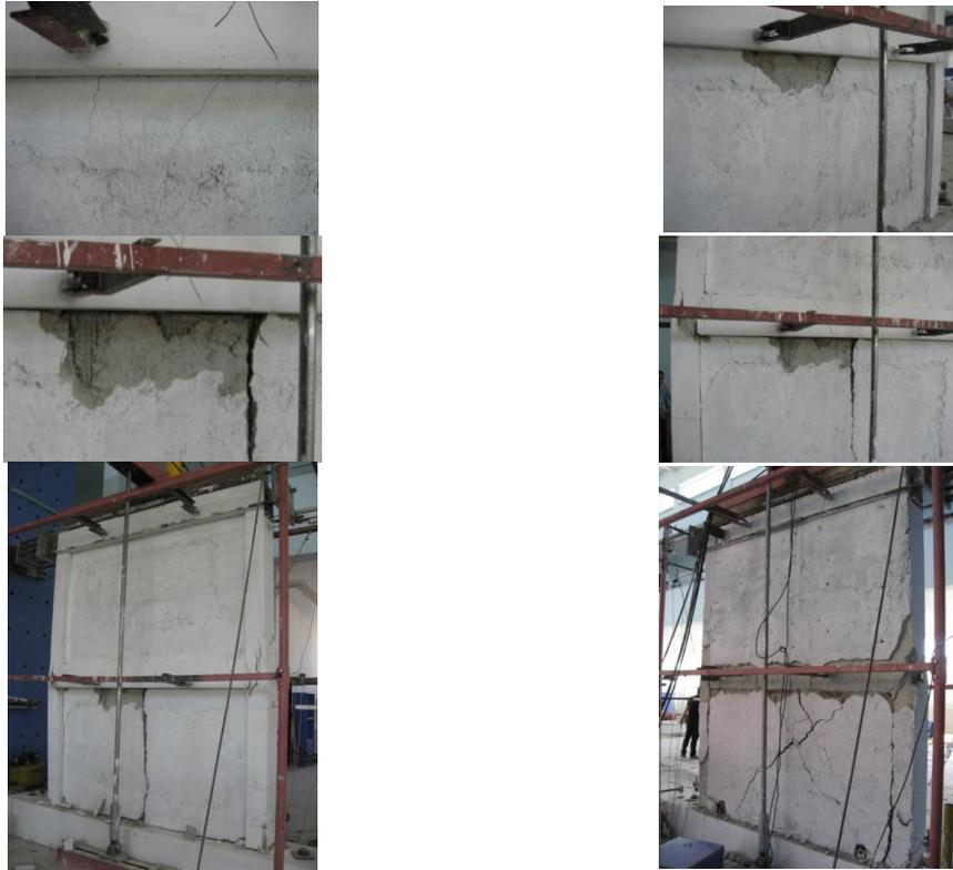
Fig. 11 Failure mode of the specimen SP3
