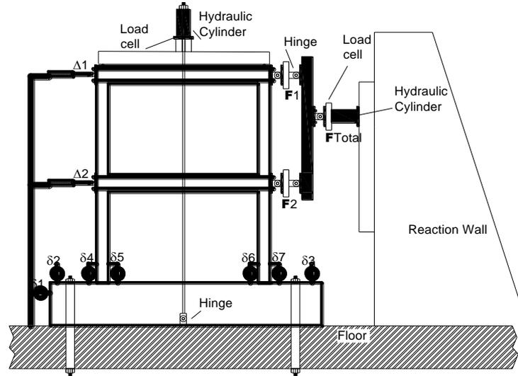
Fig. 5 Test setup, loading system, and instrumentation (Korkmaz *et al.* 2010)
