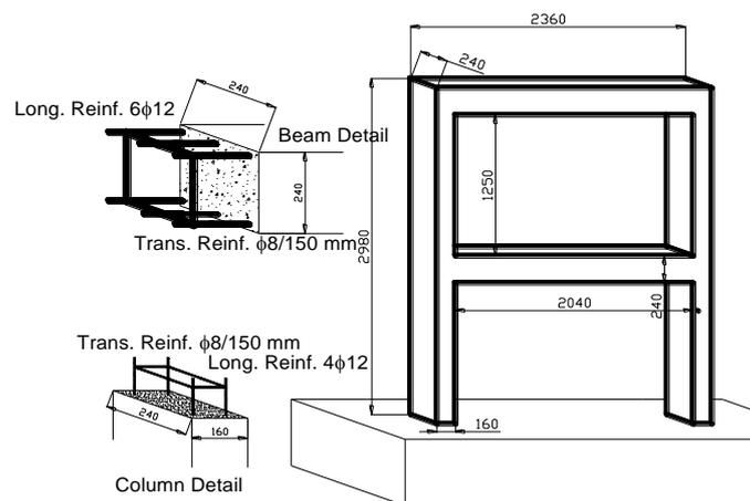
Fig. 1 Dimensions and reinforcement details of the test frames (in mm)
