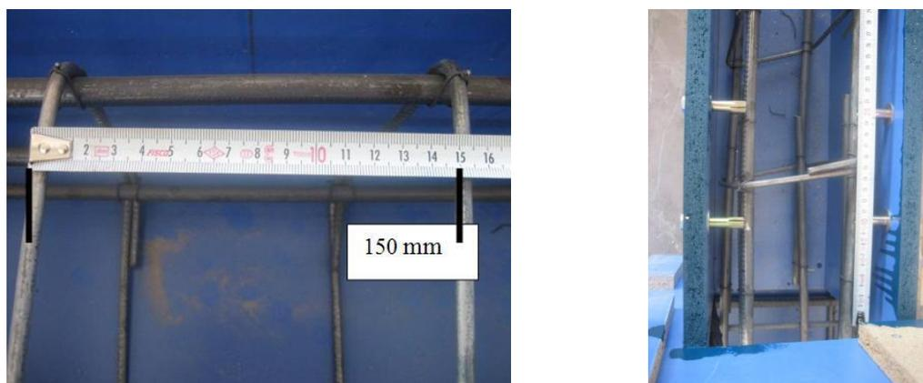
Fig. 2 Stirrups spacing and column end lap splice (Korkmaz et al. 2010)
