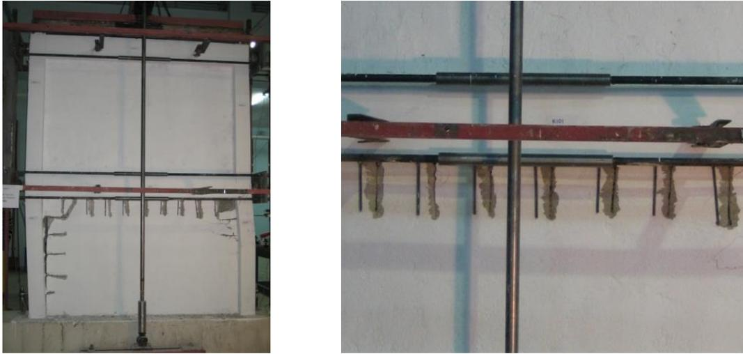
Fig. 9 Failure mode of specimen SP1 (Korkmaz *et al.* 2010)
