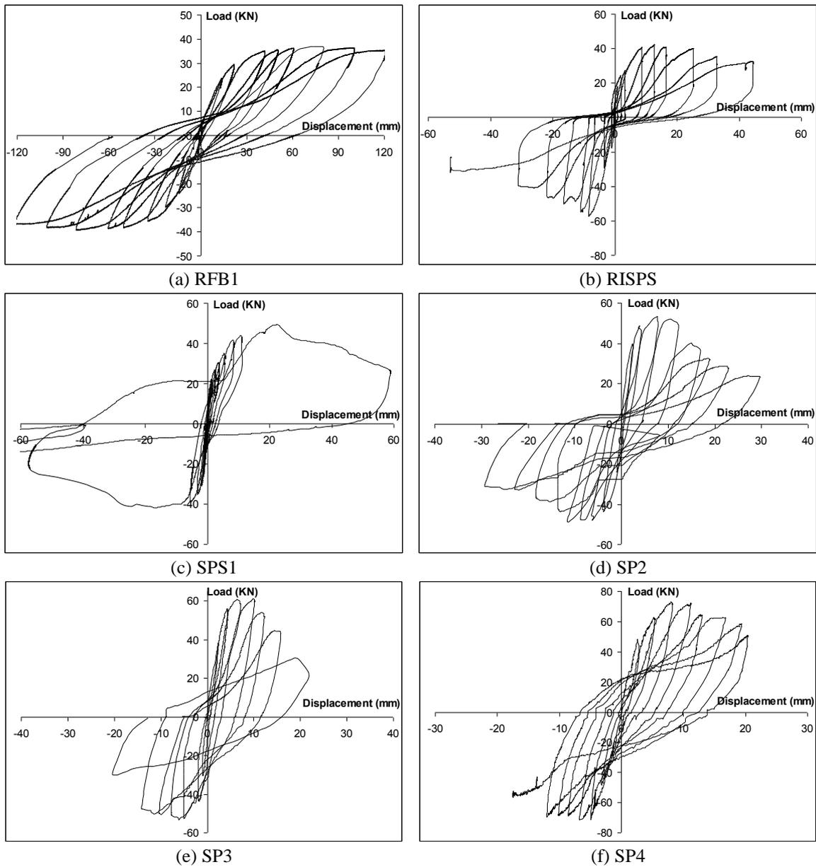
Fig. 13 Load-displacement Hysteretic curves
