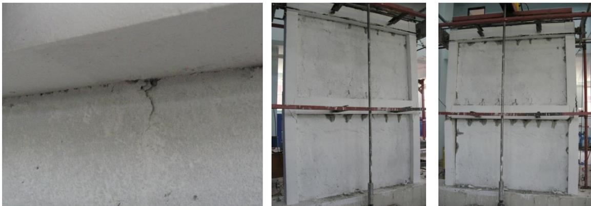
Fig. 10 Failure mode of the specimen SP2
