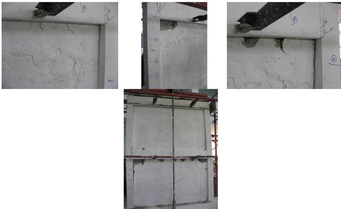
Fig. 12 Failure mode of the specimen SP4
