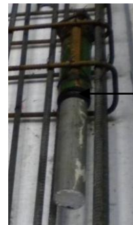
Fig. 9 Detail of specimens CFPU-2 indicating the location of U65 steel element and CFPC-2 indicating the 'gap' arrangement
