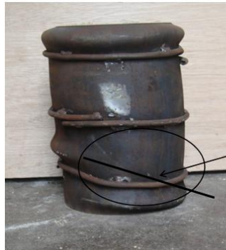
Fig. 5b Failure mode of HSCFST columns (CR20-5-168-80)
