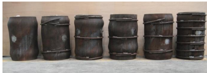
Fig. 5c Failure mode of HSCFST columns (Group no. 3)
