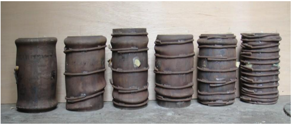
Fig. 5a Failure mode of HSCFST columns (Group no. 1)
