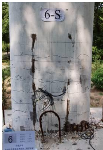
(a) Spalling at the base, SOL-6 pier
