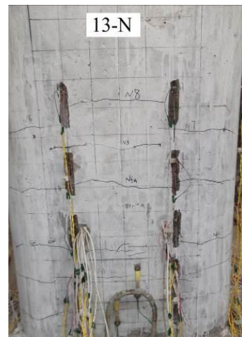
(b) Crack development, SOL-13 pier
