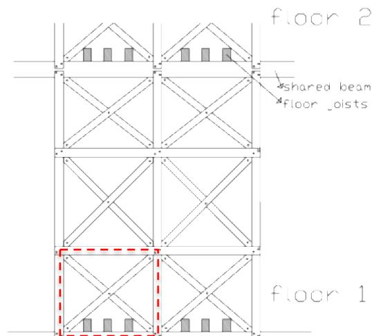
Fig. 2 Drawing of a frontal wall and its connection to the above floors (by dotted lines the modular structural scheme is marked, that is composed by the horizontal and vertical timber elements and the double diagonal bracing)
