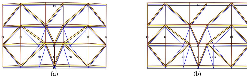
Fig. 12 Plan view of the first modal shape in Y direction in the case of a) flexible and b) rigid diaphragms, respectively and corresponding period values (in seconds) and participating mass (%)
