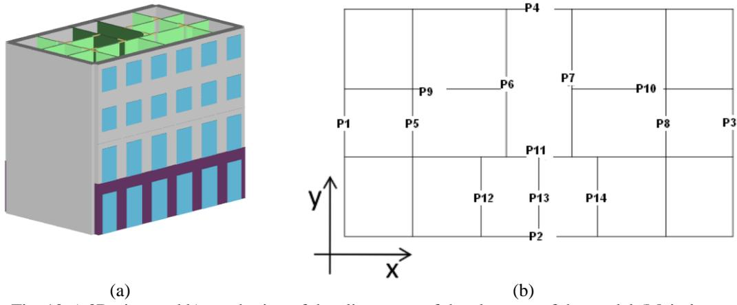
Fig. 10 a) 3D view and b) numbering of the alignments of the elements of the model (Meireles *et al.* 2012c)
