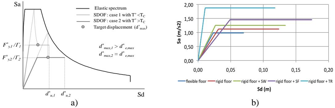
Fig. 19 a) Identification of performance point by nonlinear static procedure (Cattari and Lagomarsino 2013); b) Resulting idealized SDOF curves for the examined cases (X direction – Uniform load pattern)
