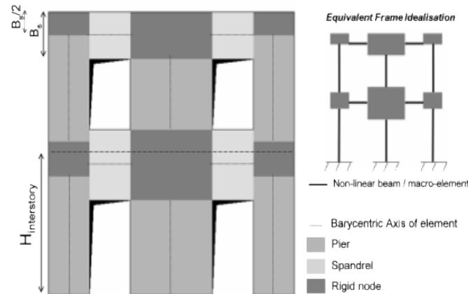
Fig. 3 Equivalent frame idealisation of a masonry wall (Lagomarsino *et al.* 2013)
