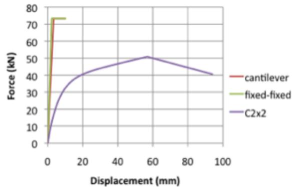
Fig. 5 Comparison between a masonry wall (cantilever and fixed-fixed) and a *frontal* wall (C2 × 2) of the same dimensions
