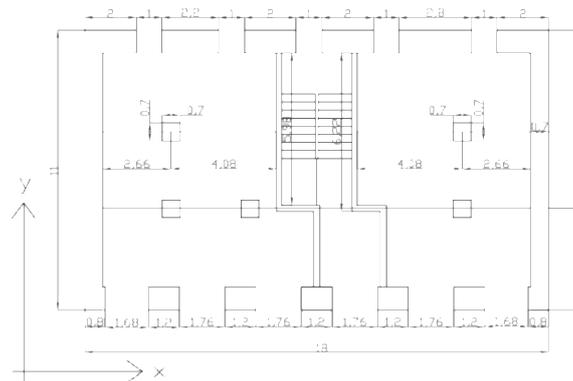
Fig. 6 Sketch of the plan view of building: ground floor – units in metres
