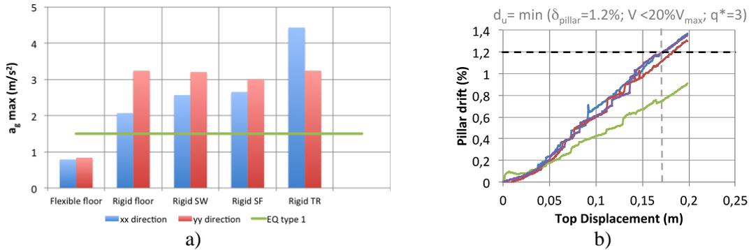
Fig. 20 a) Comparison of the seismic assessment resultant for the different configuration examined in terms of a gmax; b) evolution of drift on pillars at ground floor (X direction – Rigid floor)
