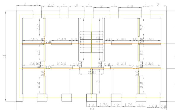
Fig. 7 Sketch of the plan view of building: upper floors – units in metres
