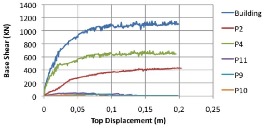
Fig. 14 Pushover curves, contribution of each wall to the base shear, X direction (rigid diaphragms)
