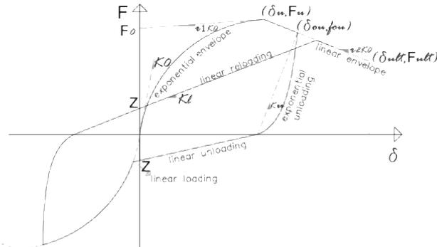
Fig. 4 Hysteresis model of frontal walls (Meireles *et al.* 2012a)
