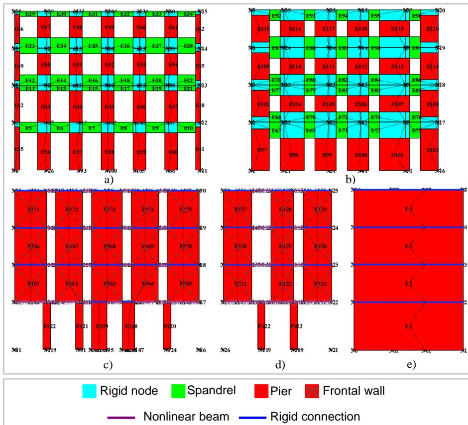
Fig. 11 Equivalent frame idealisation of: a) front façade and b) back façade (Meireles *et al.* 2012c); c) frontal walls (composed by 3x2 modular structural schemes) oriented in X -P11 and d) Y- P5 directions; e) external masonry y-y wall (P1)
