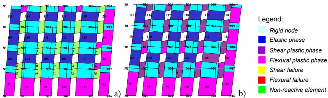
Fig. 17 Damage pattern occurred in the back façade in case of flexible diaphragms (a) and Rigid TR configuration (b), X direction (for a value of top displacement equal to 0.08 and 0.15 cm in cases a) and b) respectively)
