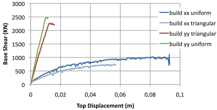
Fig. 13 Pushover curves in the two directions for both uniform and pseudo-triangular load patterns (flexible diaphragms)
