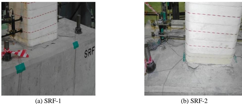
Fig. 9 Damage during the test, Retrofitted columns
