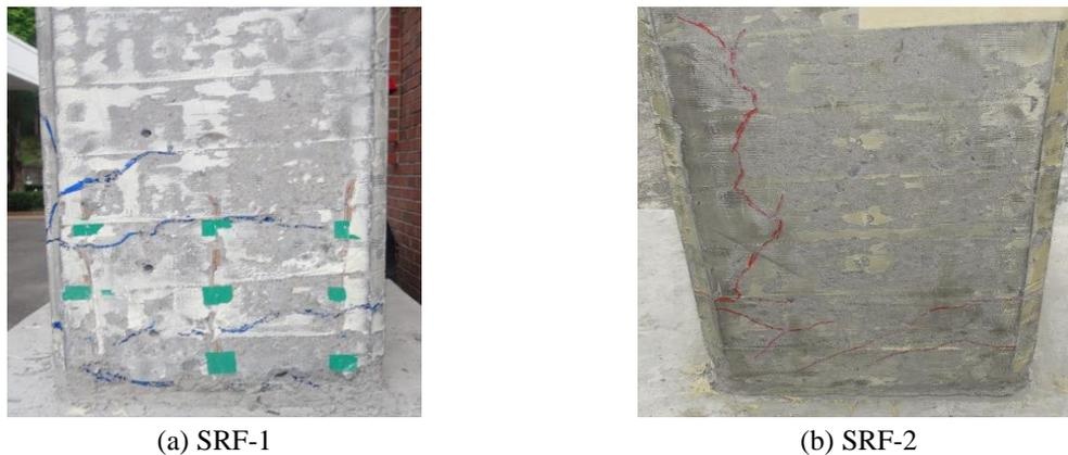
Fig. 10 Damage after tests, Retrofitted columns
