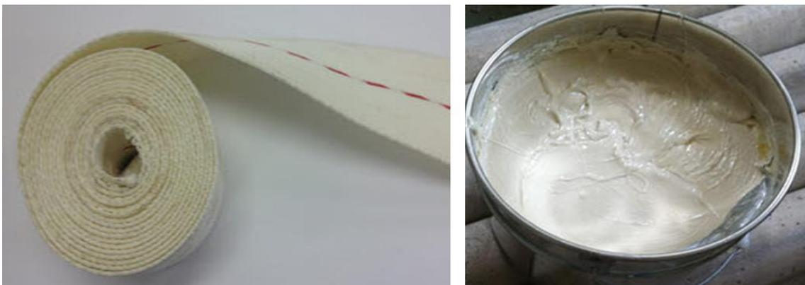
Fig. 3 SRF belt and urethane adhesive
