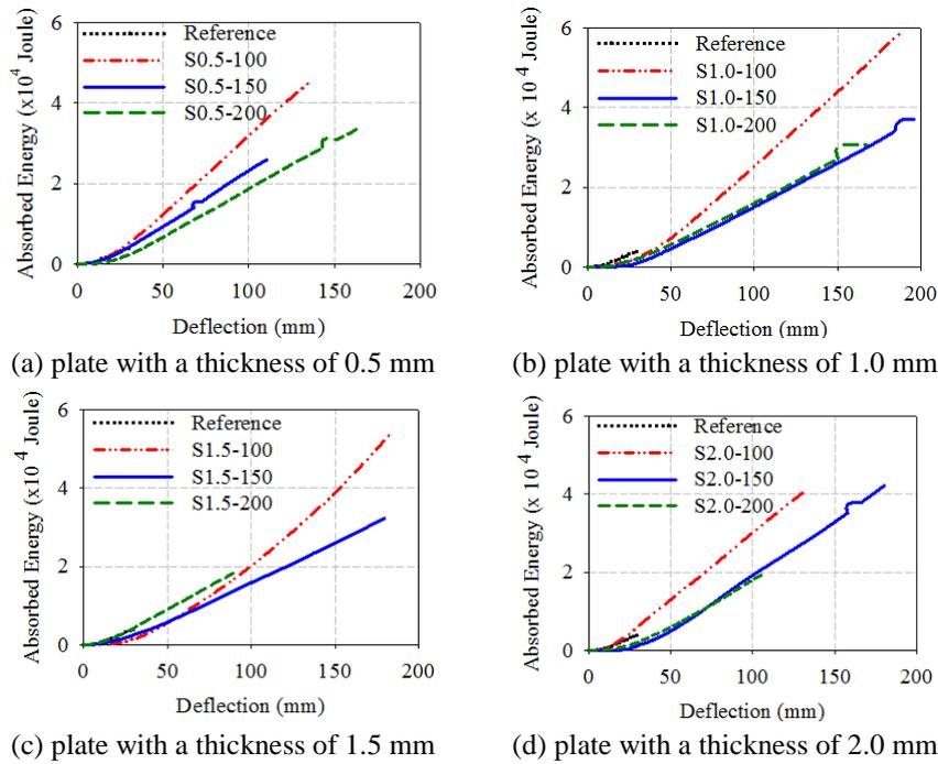
Fig. 8 Energy-deflection curves of the specimens with identical plate thickness
