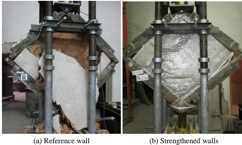
Fig. 5 Failure modes of the specimens
