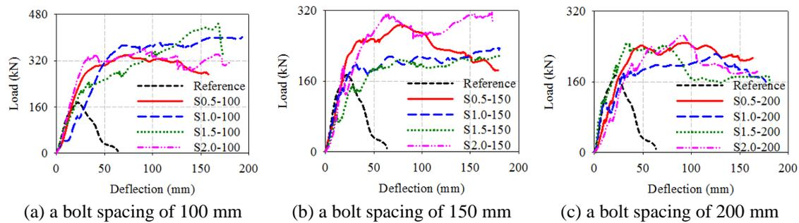
Fig. 7 Load-deflection curves of the specimens with identical bolt spacing
