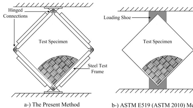
Fig. 3 Comparison of the present and ASTM E519 (ASTM 2010) methods
