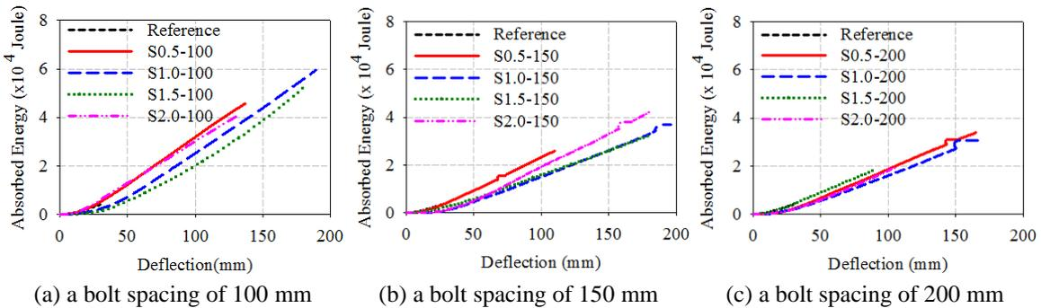
Fig. 9 Energy-deflection curves of the specimens with identical bolt spacing
