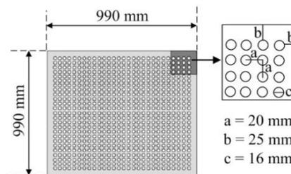
Fig. 1 Perforation pattern of the plates
