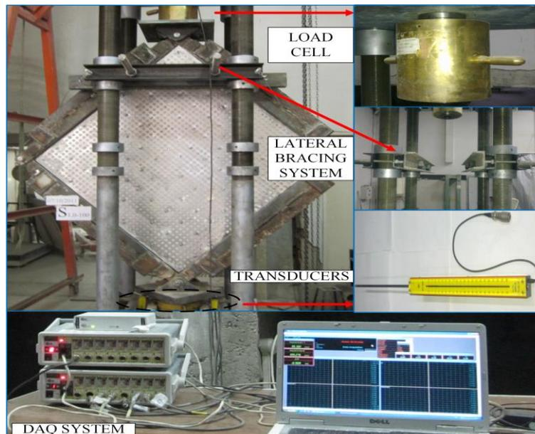
Fig. 4 Components of the test setup
