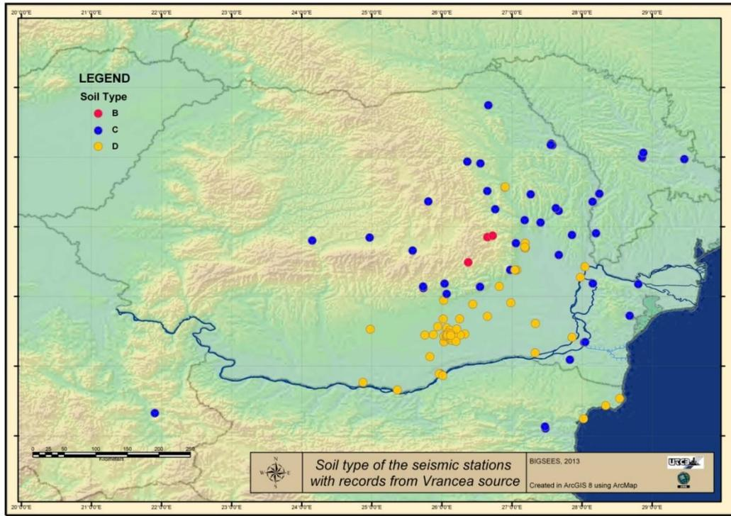
Fig. 1 Distribution of recording seismic stations and the corresponding soil conditions according to NEHRP 94
