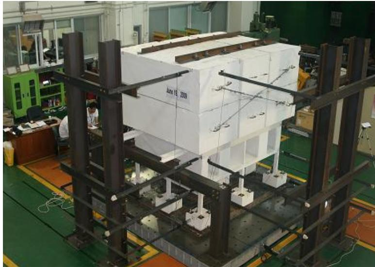
Fig. 3 Overview of earthquake simulation test set-up of the original model
