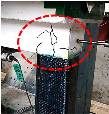
(a) Failure of joint at the top of column
