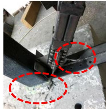
(c) Uplift of column and buckling of T angle
