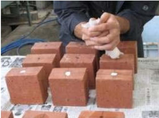
Fig. 5 Impregnant injection in drilled holes
