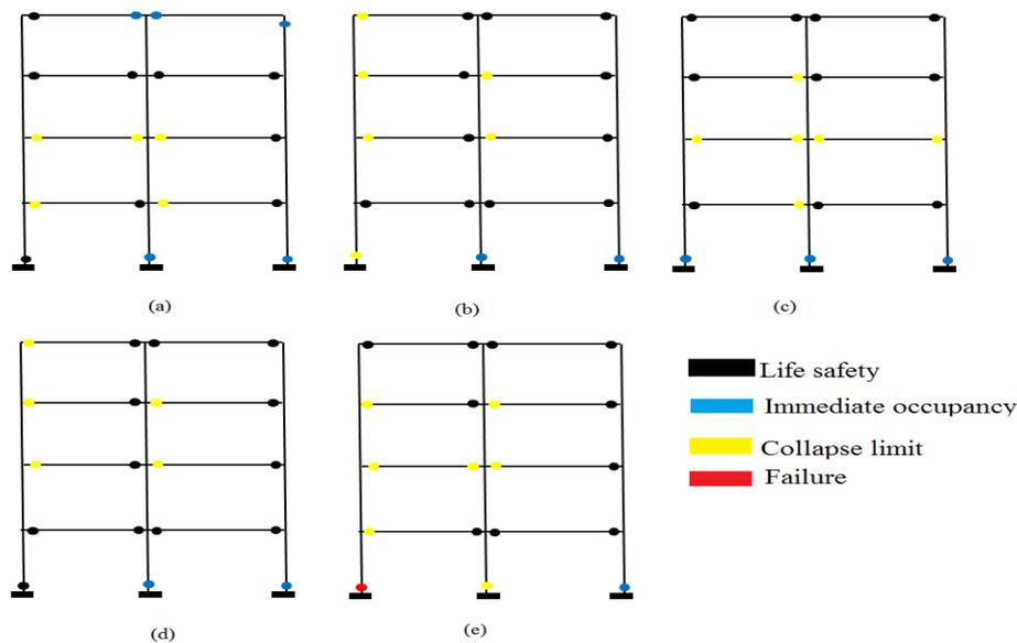
Fig. 7 Plastic hinge formations when the maximum base shear is attained: (a)S0, (b)S1, (c)S2, (d)S3, (e)S4
