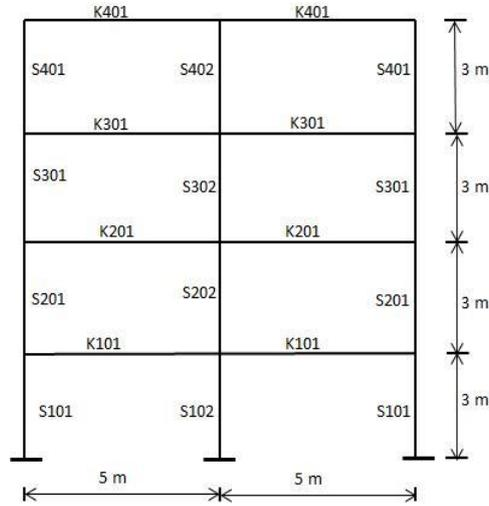
Fig. 1 Frame labeling and dimensions
