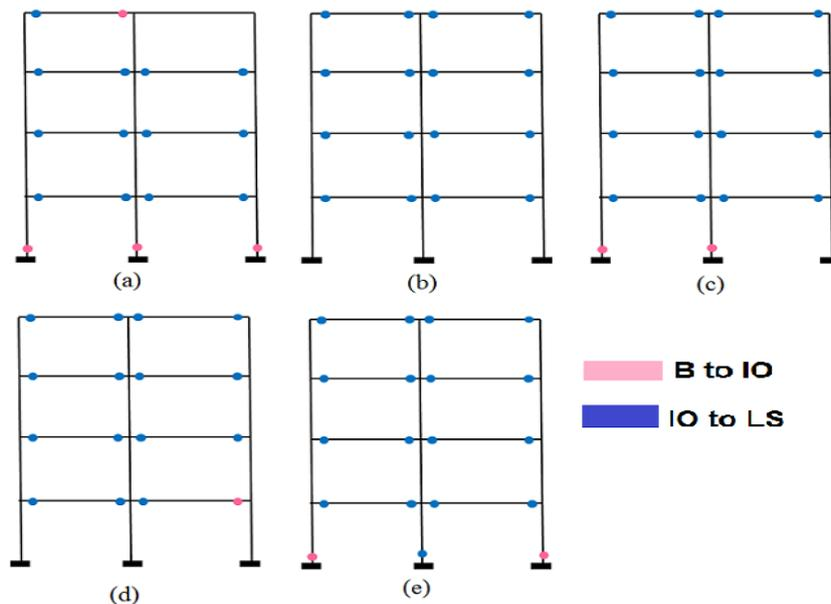
Fig. 6 Plastic hinge formation when target top displacement is attained: (a)S0, (b)S1, (c)S2, (d)S3 and (e)S4
