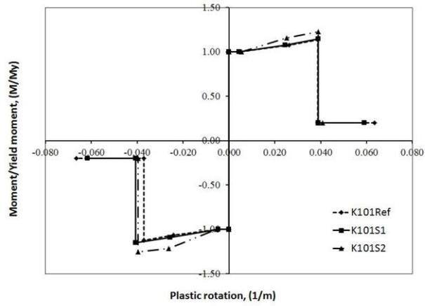
Fig. 3 Moment-plastic rotation curve for beam sections
