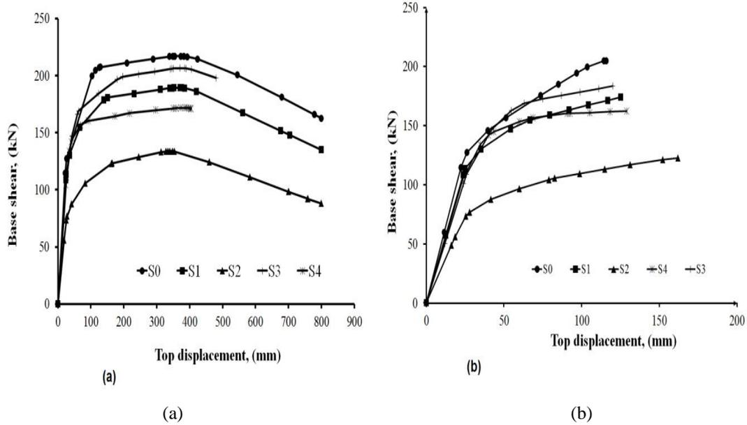
Fig. 5 Capacity curves of the frame system: (a) Up to failure and (b) Up to target displacement
