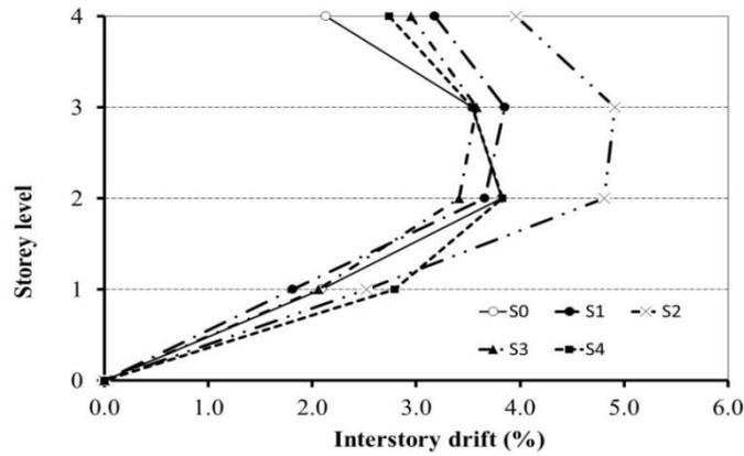
Fig. 8 Relative drifts corresponding target top displacement
