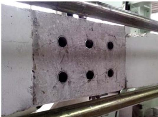
Fig. 17 Cracking at the middle of the beam (F2)
