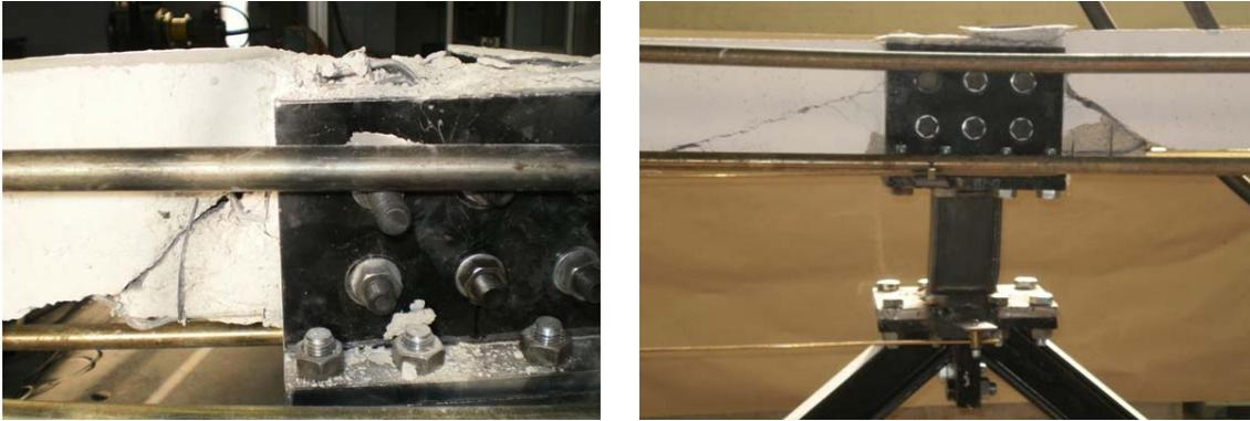
Fig. 37 Extended damage at the middle of the top beam (F5). The link did not fail
