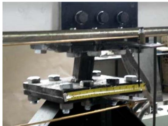
Fig. 25 Failure mode of the link element (F3)
