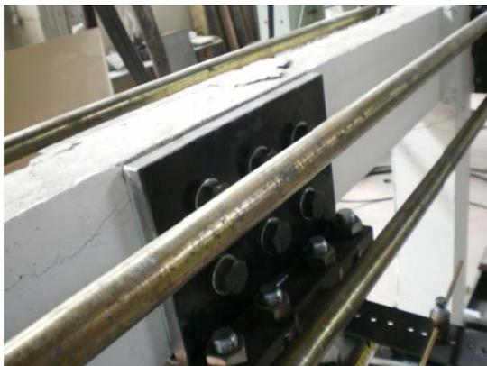
Fig. 24 Cracking at the middle of the beam (F3)
