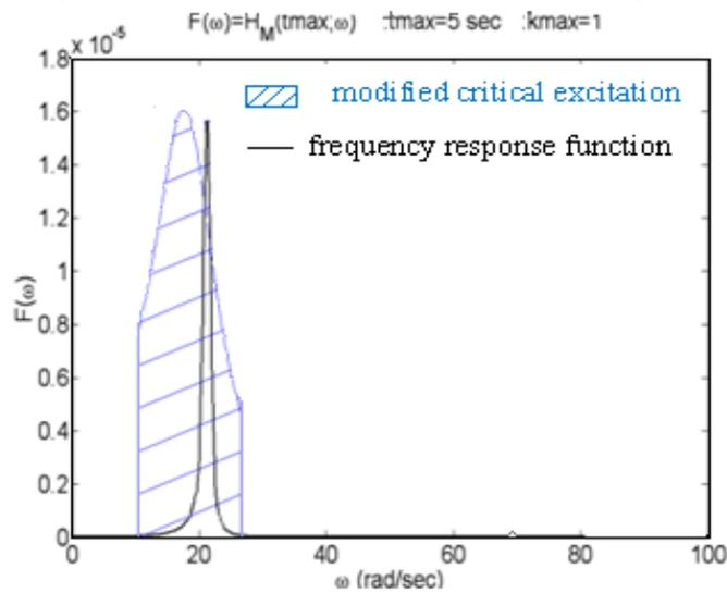
Fig. 5 Frequency content of the modified critical excitation
