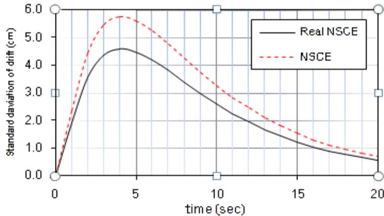
Fig. 6 Standard deviation of inter-story drift for the non-stationary critical excitation
