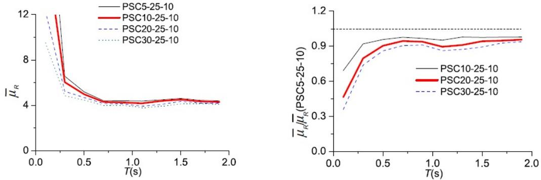
(a)  $\bar{\mu}_R$  spectra for PSC systems with different  $\alpha$  values (b) Ratios of  $\bar{\mu}_R$  for PSC systems with different  $\alpha$  values to that of PSC5-25-10 system
