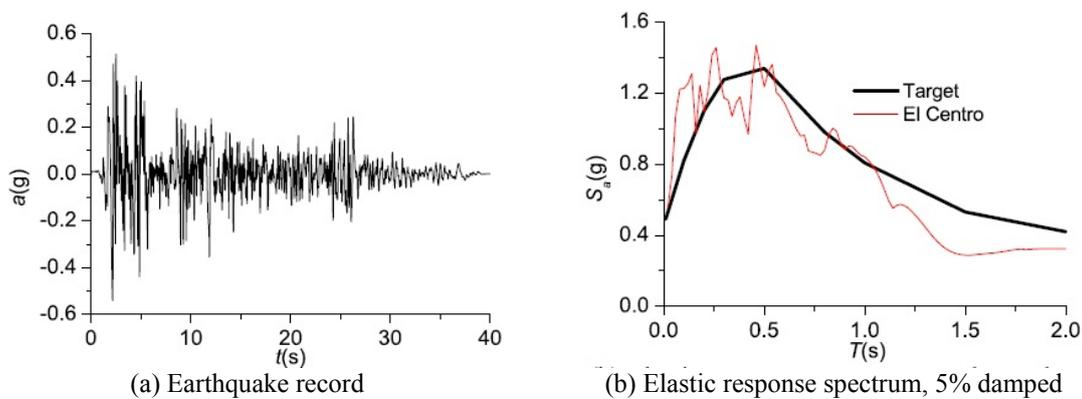
Fig. 11 Acceleration time history and elastic response spectrum for the scaled 1940 El Centro record
