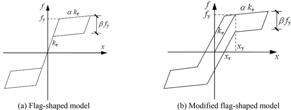
Fig. 1 Hysteretic model of (a) self-centering and (b) partially self-centering systems
