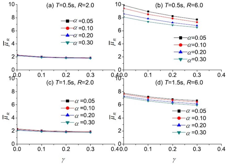
Fig. 8 Effect of combined change of  $\alpha$  and  $\gamma$  on  $\bar{\mu}_R$  ( $\beta=0.25$ )
