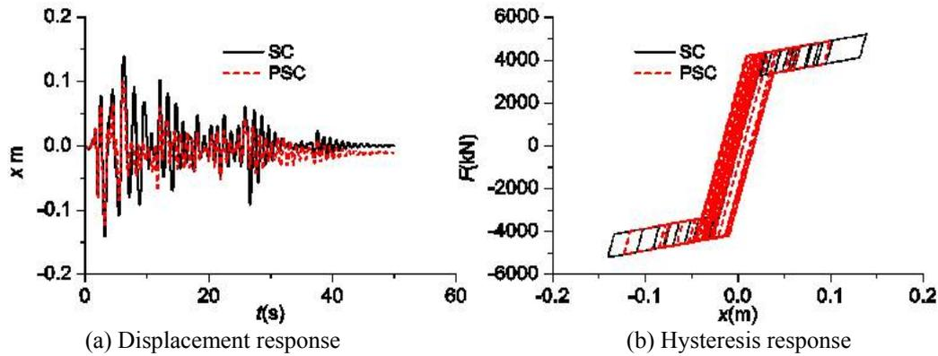
Fig. 12 Responses of the SC and PSC systems subjected to the scaled 1940 El Centro record ( $T=1.0$  s,  $R=6.0$ ,  $\alpha=0.05$ ,  $\beta=0.25$ )
