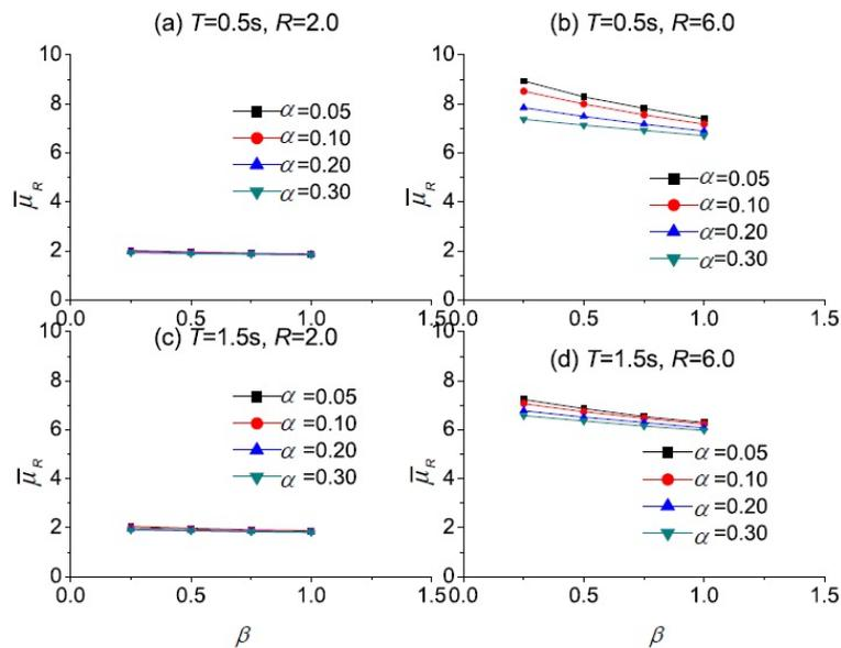
Fig. 7 Effect of combined change of  $\alpha$  and  $\beta$  on  $\bar{\mu}_R$  ( $\gamma=0.10$ )
