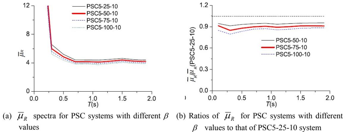
Fig. 5 Effect of  $\beta$  on  $\bar{\mu}_R$  spectra ( $R=4.0$ )
