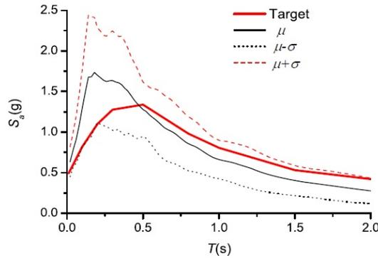
Fig. 2 Elastic response spectrum (spectral acceleration) of the 192 scaled earthquake records
