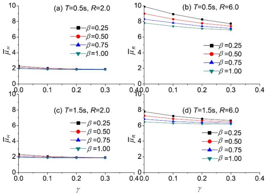
Fig. 9 Effect of combined change of  $\beta$  and  $\gamma$  on  $\bar{\mu}_R$  ( $\alpha=0.05$ )
