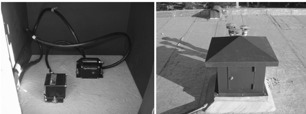
Fig. 20 External accelerometers with metal protection
