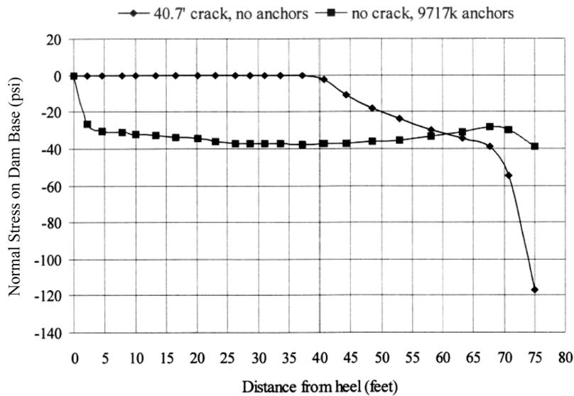
Fig. 5 Normal stress distribution on the base of the dam, with and without anchors: concrete-rock model
