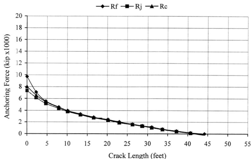
Fig. 4 Anchoring force requirement vs. crack length: concrete-rock model
