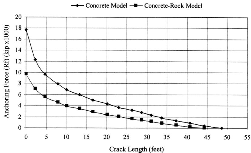
Fig. 6 Anchoring force requirements ( $R_f$ ) for the concrete and concrete-rock models
