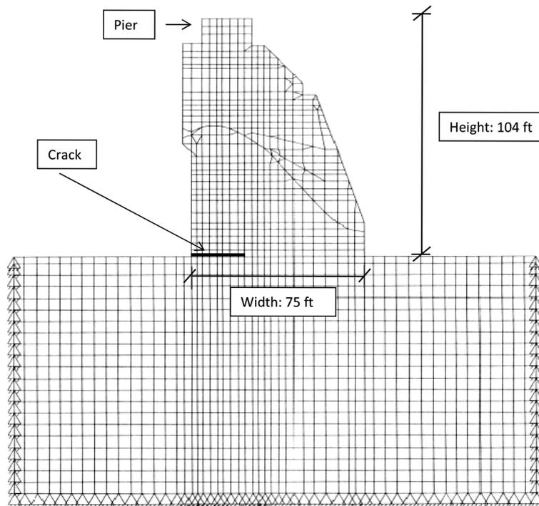
Fig. 2 Finite-element mesh and support conditions, concrete-rock model
