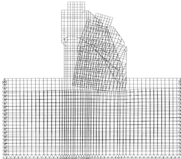
Fig. 7 Deflected shape: concrete-rock model
