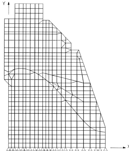
Fig. 1 Finite-element mesh and support conditions: concrete model
