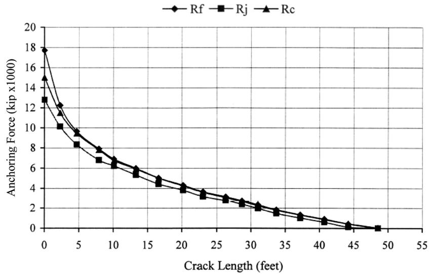
Fig. 3 Anchoing force requirement vs. crack length: concrete model
