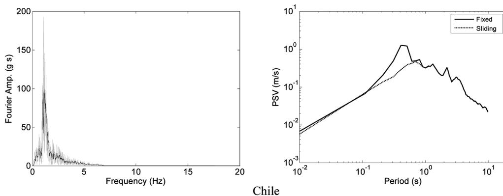
Fig. 6 Smooth Fourier amplitude spectra of different recorded and artificial accelerogram and corresponding PSV response for fixed and isolated model
