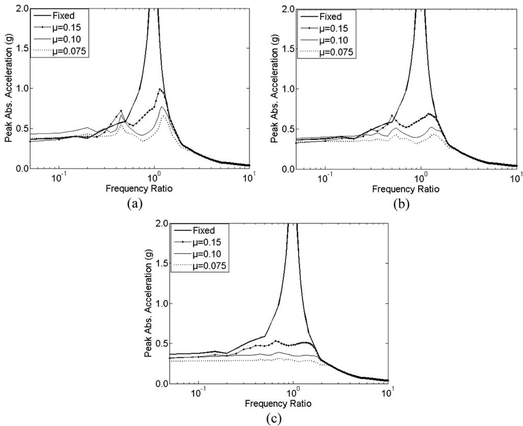
Fig. 2 Peak absolute acceleration response of the roof mass versus frequency ratio for MR=1 (a), MR=2 (b) and (c) MR=5
