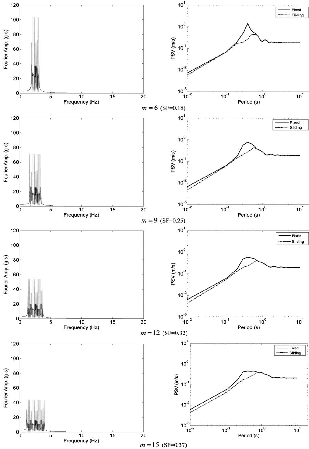
Fig. 4 Smooth Fourier amplitude spectra of different shape factor ground excitation and corresponding 5% damped PSV response for fixed and isolated model
