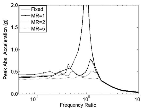
Fig. 3 Peak absolute acceleration response of the roof mass versus frequency ratio for different mass ratios ( $\mu = 0.1$ )
