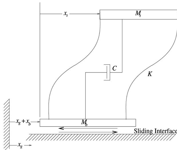
Fig. 1 Mathematical model for system with a non-sliding and sliding mode
