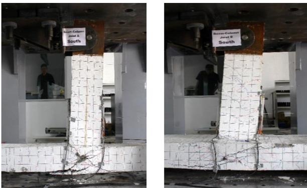
(a) BCJ-A specimen at a 5% drift ratio (b) BCJ-B specimen at a 7% drift ratio
