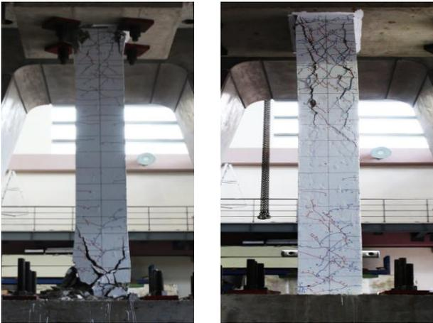
(a) C-A specimen at an 8% drift ratio (b) C-B specimen at a 4% drift ratio
